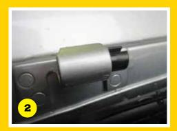
**2.** Remove the plastic slotted bushes by pushing them out of the end of the curl hinge.
