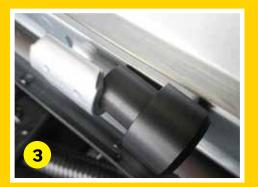
**3.** Take both halves of the new plastic bushes and try pushing them into the curl hinge on the bulkhead. The flat section of the bush goes flat against the bulkhead.
