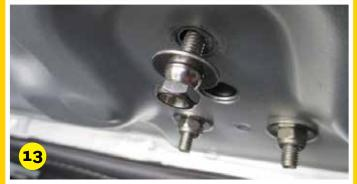
**13.** Check alignment of the bonnet and that it closes OK. Adjust hinge positioning as required. Tighten the hinge fixings on the underside of the bonnet.
