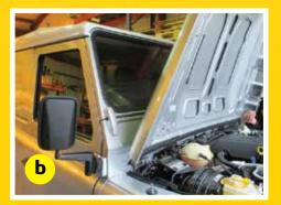
**1a & b.** Push down the car aerial. To remove bonnet from the Defender, lift the bonnet to an almost vertical/upright position. With a person at each corner the bonnet will now lift upwards and out of the plastic slotted bushes within the bulkhead hinges. Set the bonnet aside but do not fit the new security hinges to the bonnet just yet.
