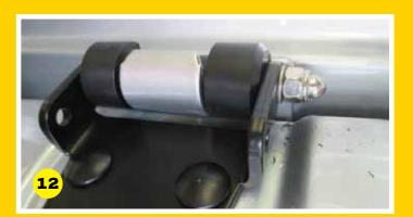
**12.** Smear some of the grease onto the exposed bolt threads and fit the nuts. Alternatively you could use a Loctite thread-lock solution as an additional security measure.
