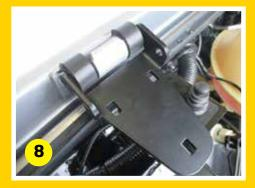
8. Offer up the bonnet hinges to ensure the bush fits within the two hinge bracket tabs.
