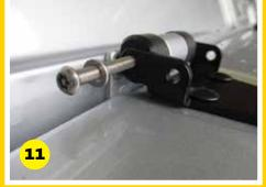
11. Offer the bonnet hinge tabs up to the plastic inserts and insert the M6 security fasteners all the way through the hinges.
