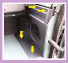
The panels fix in place using the screws provided. Drill and screw the fixings into the bodywork (bodytub capping & wheelarch) in the locations as illustrated by the arrows above.
