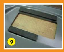
Offer up the centre section of the roof console ensuring the front edge of the console wraps around the front of the headlining as illustrated.
