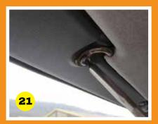
Check the alignment of the fixings for the remaining fir-tree fasteners holes where they meet the central console section and push the remaining fasteners home.
