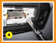
The interior light will now release from the base plate. Squeeze the plug to release wiring harness from interior light.
