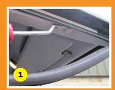
Remove the sun visors by removing fixing screws x 4.
