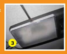
Remove interior light by unscrewing the two 8mm nuts.
