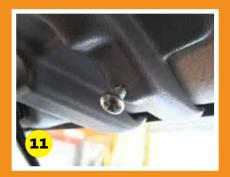
With the console held in place by the 2 x sun-visor screws you are ready to drill the holes for the firtree fasteners.
