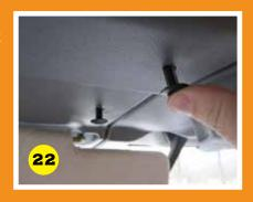
Use the remaining large fir-tree fasteners for the central shelf supports.
