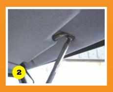
Remove interior light lens by releasing with a small flat bladed screwdriver.
