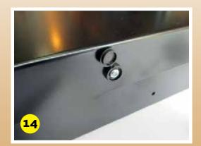
Fix the MUD Cubby Box Locker into the vehicle using the  $4 \times M6 \times 25$ mm socket button fixings and large washers.
