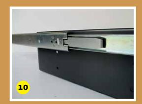
Fasten the drawer slides to the locker base using the upper most fixing holes on the side of the locker base.
