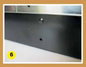
The locking mechanism on the hinging Cubby Box locker is pre-installed. The sliding Cubby Box Locker requires the locking mechanism fitting into the MUD Cubby-Box Locker. Thread the locking mechanism through the hole in the front of the box and secure using the large nut. The locking tab should point vertically upwards when in the locked position.
