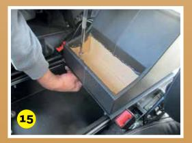
Position the divider plates within the MUD Cubby Box Locker to suit your requirements and fix in place using the plastic fixing rivets. Insert your pre-cut rubber matting.
