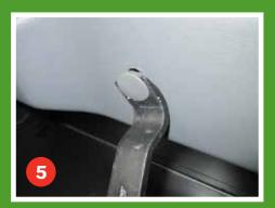
Remove the 3x Fir Tree fasteners securing the 'window' trim including the 1x Fir Tree fastener at the very front of the interior trim. Ideally use a trim removal tool to remove the Fir Tree Fasteners to prevent damage to the trim.
