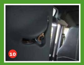
Thread the seat-belt through the slot in the interior trim to allow you to remove the trim from the vehicle.
