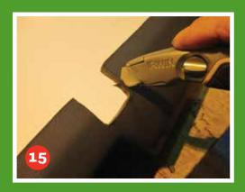
Increase the width of the notch in the trim with a sharp blade or a junior hacksaw. Trim a little at a time so that you end up with a neat snug fit around the MUD Utility Wagon trim centre rib.
