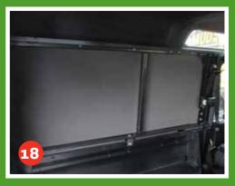
The MUD Utility Wagon trim will sit into the back of the factory trim whilst you install it in the vehicle.
