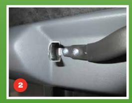
Remove the grab handle from the interior trim. The fixing screws are concealed by the flip-up lid on the handle.
