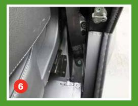
Undo the seat-belt fastener with a 17mm socket/spanner.
