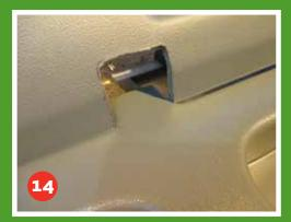
The notch in the centre of the factory trim needs to be enlarged to allow the MUD Utility Wagon trim to sit down within the notch so that it sits flush on the back of the window opening.
