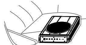
2. Make sure there is sufficient air circulation around the intended mounting location.
