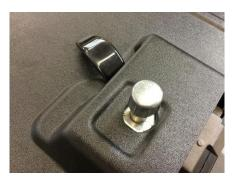
Position the nets within the recess on the trims and use a 2.5mm drill or bradawl to create the net fixing holes. Fix the nets in place using the small self-tapping screws. Push the screw cap into place. Use the head of a screwdriver if the screw-caps are a tight fit.
