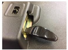
On the earlier Series handles with the push-and turn locks the only trimming required to the trim is to create a hole for the lock to protrude through the door panel. We recommend using a hole-saw with a minimum diameter of 27mm to clear the lock handle. Alternatively, remove the rectangular recess as described above for the anti-burst style handles.
