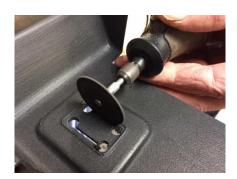
Removing the area around the handle opening, indicated in yellow in the picture below will provide clearance for the anti-burst door handle mechanism. The range of movement between handles varies greatly. We recomend measuring 10mm inwards in the area indicated below and remove the material.
