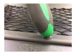
To fix the trim to the door, drill through the pre-drilled holes around the outside of the trim into the door frame with a 5.5mm drill. Fix the trims in place on the doors using the fir-tree fasteners.
