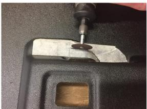
Once the lock and handle mechanisms moves freely through their full range of travel without interference, finish off the trimmed areas with a file to tidy any rough cut edges.
