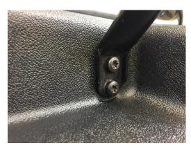
The trim is secured to the door by fasteners in the locations illustrated in red below. Be careful when prising the old trim away from the door so as not to damage the fragile trim clips (LR Part# EYC000230). When you have released all eight fasteners around the outside edge of the door frame, the central fastener is located within a slotted moulding on the door. To release the panel from the door, slide the entire trim panel downwards.
