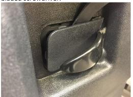
Remove the door grab handle. The grab-handle is secured by 4 x TX25 Torx fasteners.
