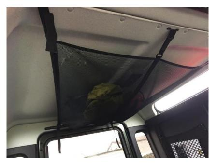
On vehicles with a trim above the rear door, align the central footman loop with the grab handle fasteners. This way you can be sure to hit the gutter section that the grab-handles also screw into.
