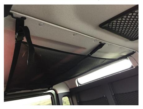
Front Net Mounting 90: Align the footman-loops with the row of plastic trim rivets securing the headlining into the roof directly above the front seats.
