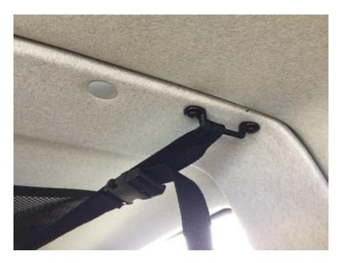
Position the front footman loops as far apart as possible at the point where the internal roofline begins to curve. Use a 2.5 mm drill bit to drill the fixing holes for the footman-loops.
