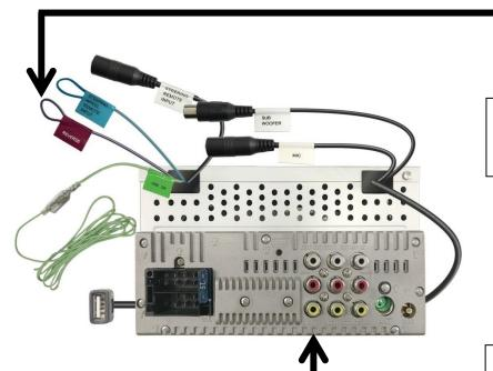
Reverse input from Piggy-Back loom/ Reverse lamp connects into Purple/White wire marked 'Reverse'
