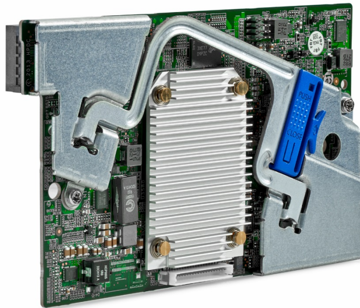
HPE Smart Array P244br Controller
