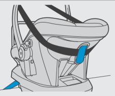
Fit tether into blue guide at rear of shell whenever the restraint is used in a vehicle.
