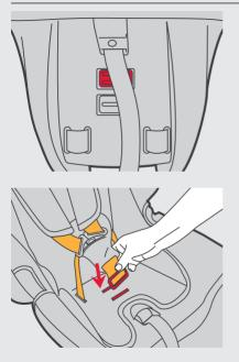
PURPOSE: the crotch strap can be adjusted forward for bigger children. When purchased the crotch strap will be in the rear position. Only move it to the forward position when the child weighs more than 7kg. Typically this is when the harness is in the top slots.
