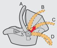
Any handle position is suitable for use in the car.
