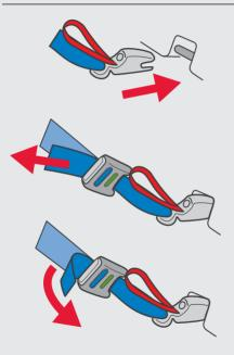
If necessary release the adjustors and extend enough web through them so that the ISOFIX compatible connectors can reach the anchor points.
