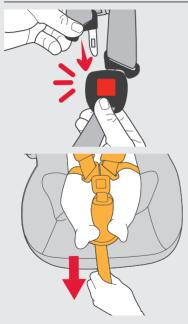
Insert buckle tongues into the buckle, when the second tongue is engaged until you will hear a "click". If you do not hear a click recheck if the tongues are secured correctly. If the tongues do not secure correctly **see page 43** for buckle cleaning instructions.
