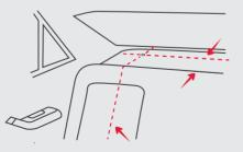
WARNING: CHILD RESTRAINTS MUST NOT BE ATTACHED TO UNSOUND METAL OR TO WOOD, OR SYNTHETIC STRUCTURES. WHEN DRILLING THE 9 MM HOLE DO NOT DRILL THROUGH FUEL LINES, FUEL TANKS, ELECTRICAL WIRING, OR RADIO SPEAKERS. WEBBING STRAPS MUST BE PROTECTED FROM SHARP CORNERS AND EDGES.
