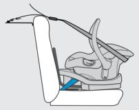
Pull to increase tension, press adjuster button to loosen.
