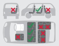
Do not install the child restraint on a vehicle seat that faces either sideways or to the rear of the vehicle.
