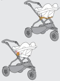
IMPORTANT: SECURELY ATTACH the child restraint to the stroller and LIFT IT UP TO CHECK that it is attached.
