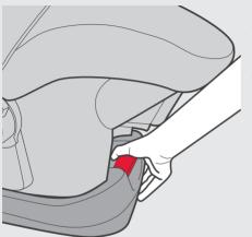
Pull up on the red release lever at the back of the base, and lift the child restraint out.
