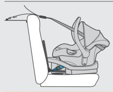
NOTE: in some installations the shape or softness of the vehicle seat cushions may prevent the indicators from showing fully green even when the straps are pulled tight.
