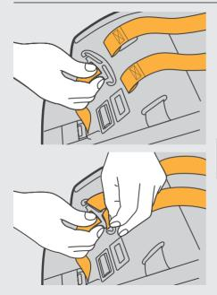
From the rear of the seat, secure the harness strap onto the splitter plate.
