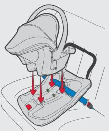
Put the child restraint rear facing on the base, and press it downward.
