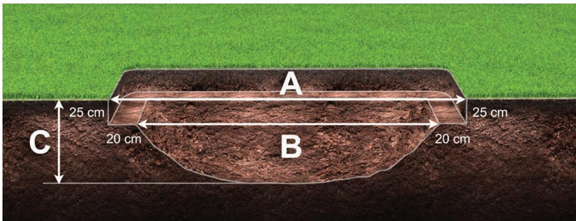
The hole should not accumulate water (in which case the drainage is necessary) and it should be possible to clean during maintenance.
