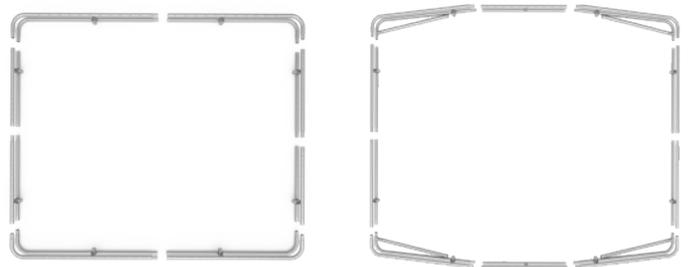
Please note: On the long sides, the frame will appear to bow outwards - this is by design. When the springs are attached the frame will pull inwards, but always have a slide outward bow.
