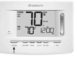
to set your heat or cool temperature within 3° F of each other. If a setting is made in either heating or cooling which violates the dead band, the opposite mode will adjust up or down automatically to maintain the programmed dead band spacing.
