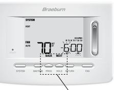
BACK and NEXT are secondary functions of the PROG and HOLD buttons.
