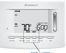
BACK and NEXT are secondary functions of the PROG and HOLD buttons.
