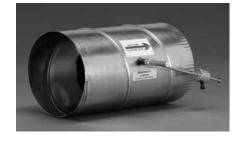
damper is lightly closed. As supply dampers close and pressure builds in the supply air plenum, the pressure pushes the bypass damper open. A simple, adjustable weight is used to properly position the damper.
