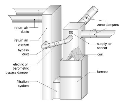
In many zoning installations it is necessary to install a bypass damper. A bypass damper will help the HVAC equipment maintain rated CFM past the heat exchangers and blower motor. If a system does not have a bypass, and only a few dampers are open, excess supply plenum pressure may be created. The result can be system limit trip-outs, excess noise, coil icing, or other problems. The bypass damper is installed in the bypass system duct.
