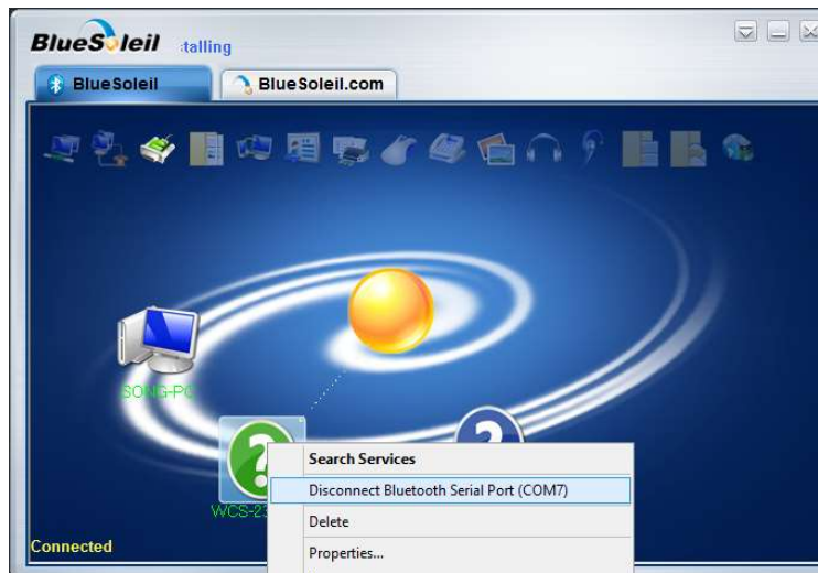
[Figure 18. Disconnect Bluetooth Device from Serial Port]
