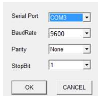
[Figure 8. WCS-232 V6.0 Setup Program Port Setting]
