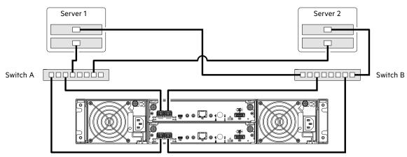
Figure 18 Connecting hosts: switch attach—two servers/two switches
