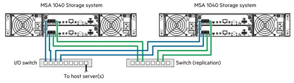
Figure 20 Connecting two storage systems for Remote Snap: multiple servers/switches/one location
