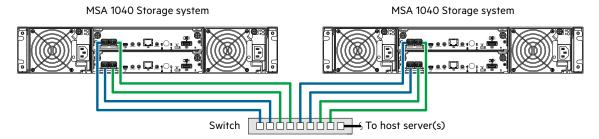
Figure 19 Connecting two storage systems for Remote Snap: multiple servers/one switch/one location
