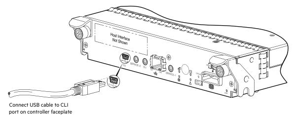
Figure 23 Connecting a USB cable to the CLI port
