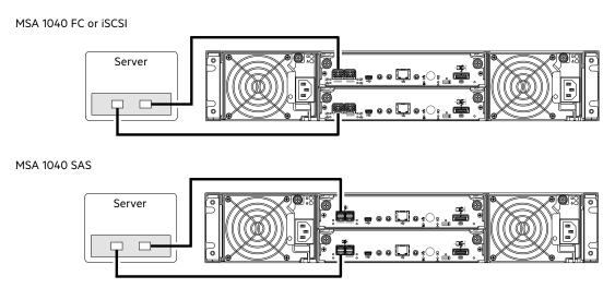
Figure 15 Connecting hosts: direct attach—one server/one HBA/dual path
