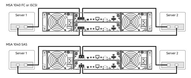
Figure 16 Connecting hosts: direct attach—two servers/one HBA per server/dual path
