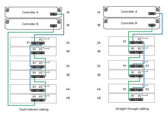
Figure 11 Cabling connections between MSA 1040 controllers and SFF drive enclosures
