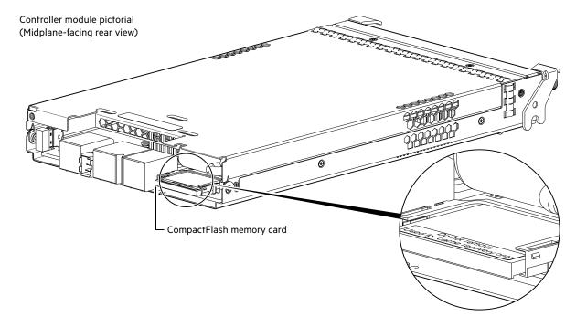
Figure 8 MSA 1040 CompactFlash memory card
