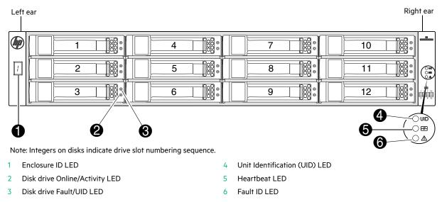
Figure 2 MSA 1040 Array LFF or supported 12-drive enclosure: front panel
