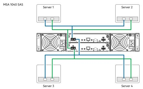
Figure 17 Connecting hosts: direct attach—four servers/one HBA per server/dual path (fan-out)
