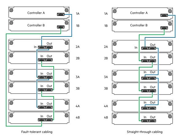
Figure 10 Cabling connections between MSA 1040 controllers and LFF drive enclosures
