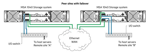
Figure 22 Connecting two storage systems for Remote Snap: multiple servers/switches/two locations
