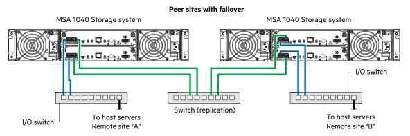
Figure 21 Connecting two storage systems for Remote Snap: multiple servers/switches/two locations
