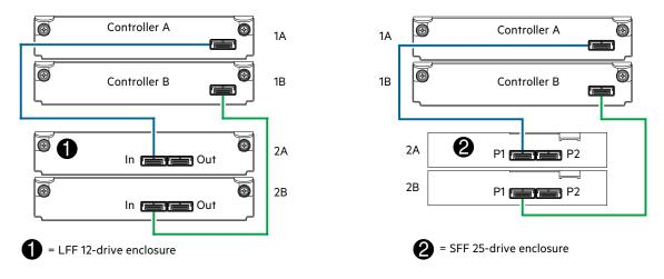
Figure 9 Cabling connections between the MSA 1040 controller and a single drive enclosure
