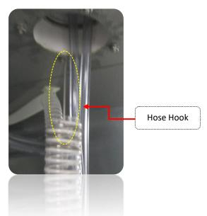
Be sure that the hose hook is correctly attached into the tower hole.
