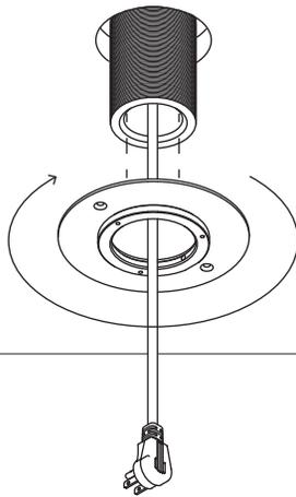
Rotating clockwise, secure the base plate onto the base column until it reaches the desired height.
