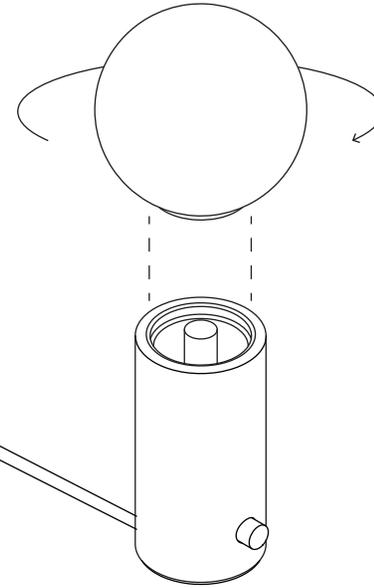
Attach the diffuser to the lamp base by rotating clockwise until fixed in place
