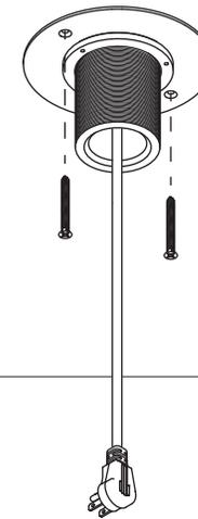
Secure the base plate onto the underside of the table by using the screws provided or screws that are appropriate for the surface.
