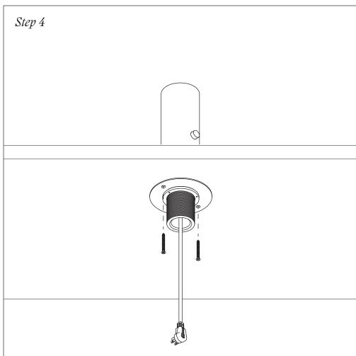
Secure the base plate onto the underside of the table by using the screws provided or screws that are appropriate for the surface.
