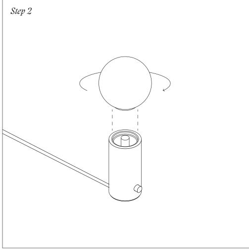
Screw the included lightbulb into the socket of the lamp base.
