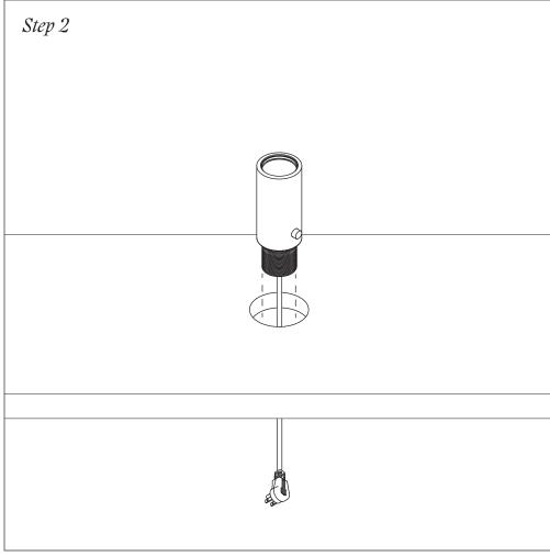
Drill out a 2 ½" diameter hole to fit the threaded base column.
