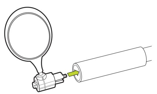
Twist knob on mirror clockwise to tighten the expanding bolt securing the mirror to the bar.
