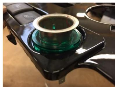
If you want to upgrade the standard Land Rover socket to a Bluesea 12v or dual USB socket, you will have to increase the original 26mm diameter hole in the panel to 28mm. The easiest way to do this is with a deburring tool. The external dimensions of the Bluesea sockets drop neatly into the recess in the Puma dashboard.
