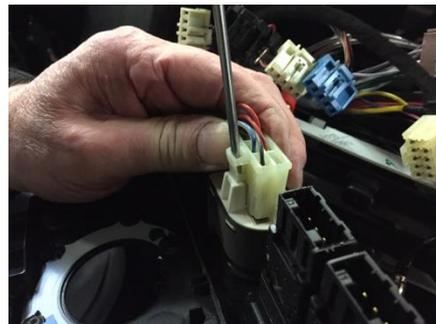
With the dashboard free from the vehicle, you can transfer the switches and controls across to the new fascia panel.
