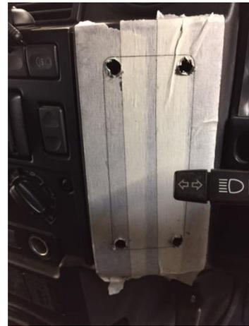
Once you've done that then it's just the time-consuming matter of extending your switch wiring to the new switch locations within the relocation panel. The switch apertures within the relocation panel are not keyed to any particular switch so play around with different positioning of the switches within the relocation panel to create extra wiring length where needed.
