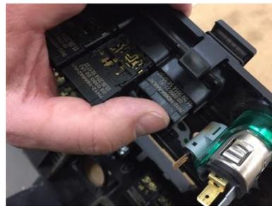
The cigarette lighter socket is the trickiest part to remove. It is very common for the plastic bulb holder to become hard and brittle due to heat from the bulb. This often results in the locating tabs breaking when you try to release them. Providing the earth contact maintains contact with the body of the 12v socket, a wrap of insulating tape to hold the bulb holder to the socket will ensure the socket will continue to illuminate.
