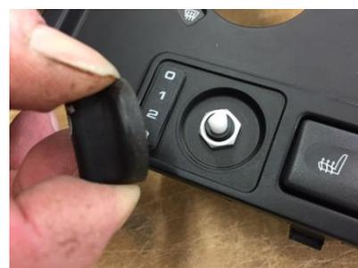
The clock is held in place with 4 x TX15 screws Using a magnetic screwdriver makes their removal and refitment easier. With the clock removed, release the securing tab on the hazard switch with a thin bladed screwdriver.
