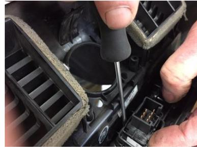
To release the electric window switches, squeeze the release tabs top and bottom.
