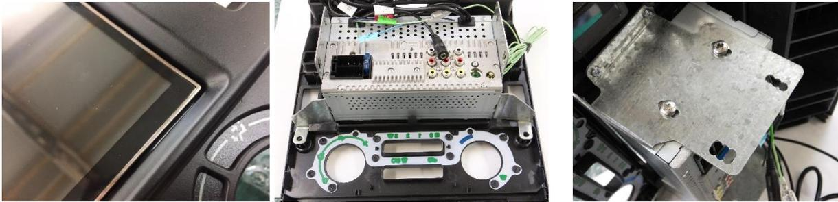
You'll notice the installation pictures show a mech-less head unit with a shallow overall depth (JVC KW-M745DBT). We very strongly recommend selecting a shallow depth mech-less (no CD player) Double DIN head unit for your new fascia. This will save you much of the time and hassles normally associated with Defender Double DIN installations.
