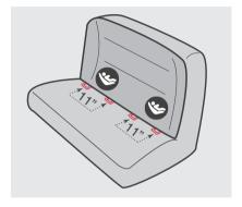
LATCH may be used for spacing larger than 11" ONLY if your vehicle manufacturer allows it.
