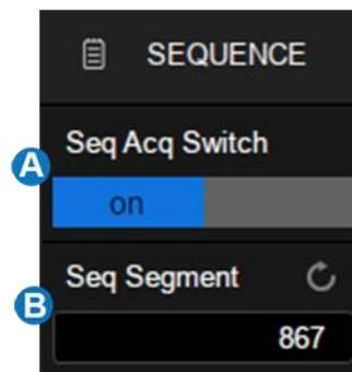
Sequence mode is a fast acquisition mode, which divides the memory depth to multiple segments (up to 90,000), each of which stores a single shot. In sequence mode, the oscilloscope only acquires and stores data without processing and displaying, until the specified segments are acquired. As a result, the dead time between trigger events is minimized, thus greatly improving the waveform update rate. If sequence mode is
