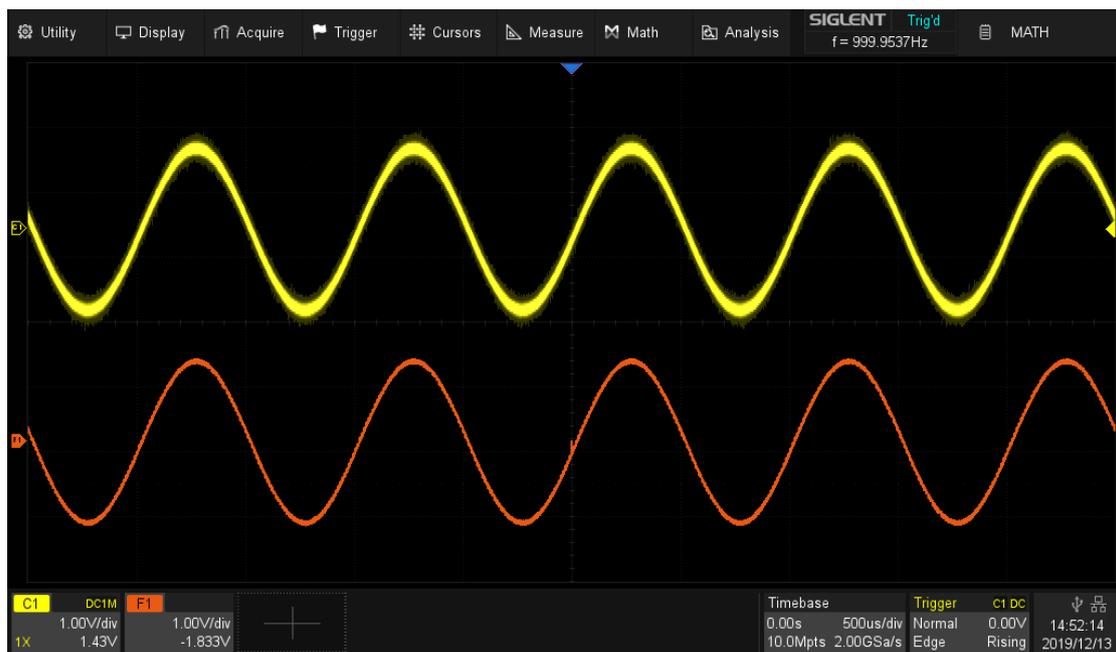
**Note:** Average acquisition is only valid for periodic signals, and it is important to ensure that the waveform is triggering in a stable way when using average mode.
