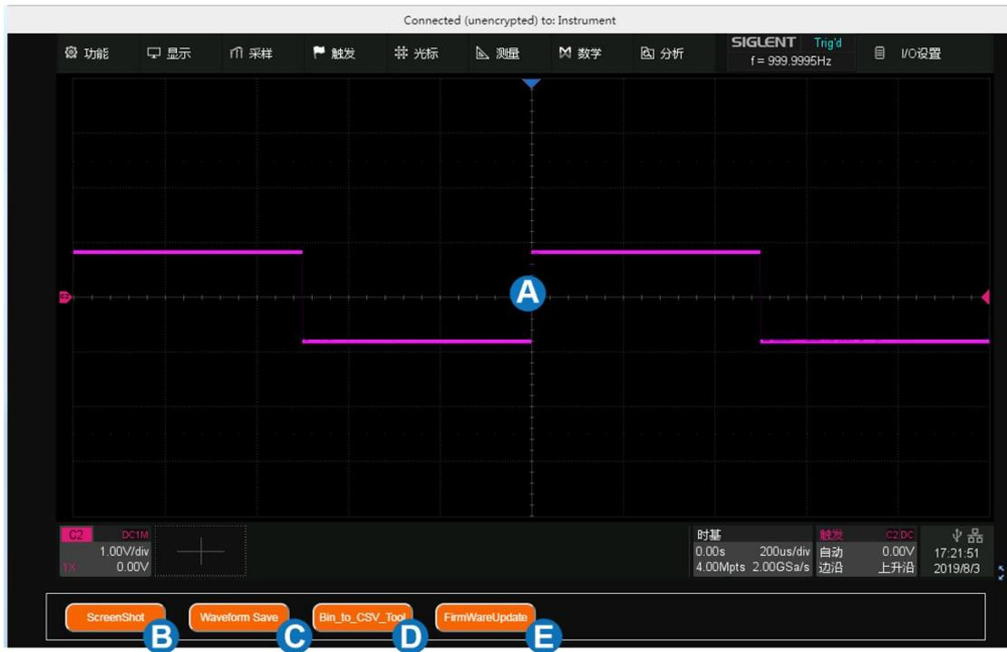
A. Display and control area of the instrument. The display in this area is a copy of the instrument display. Using the mouse to operate in the area is equivalent to directly operating the touch screen display of the instrument.
