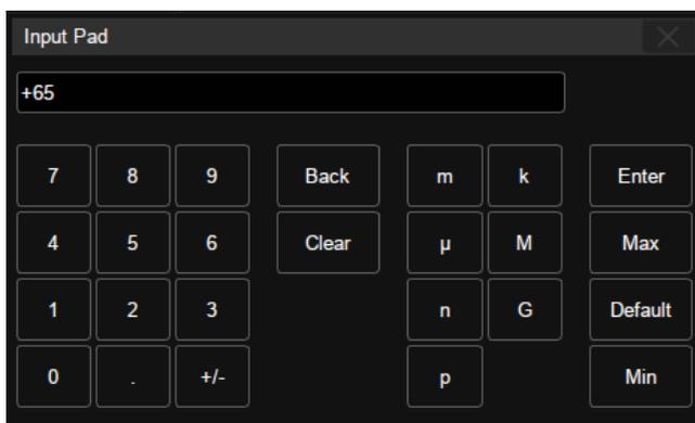
Let's use the operation of setting the "deskew" of a channel as an example: If the expected value is 65 ns, input "65" on the virtual keypad, and then choose the unit n to complete the operation. On the virtual keypad, touching the button Max, Min, and Default quickly set the parameter to its maximum, minimum and default values.
