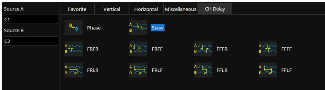
In the parameter selection area, the channel corresponding to *Source A* is specified first, and then the channel corresponding to *Source B*. Finally, the measurement parameter is selected. For example, to activate the skew between C1 and C2, you can follow the following steps:
