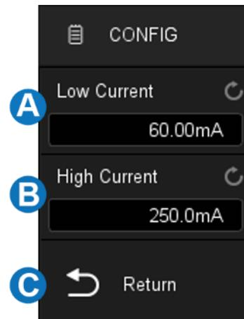
**Note:** low current value and high current value are used to calculate the trigger level and adjust the oscilloscope vertical scale. After the load changes, the current value changes from low to high (or from high to low), and the oscilloscope triggers and performs to measure the transient response stability time.
