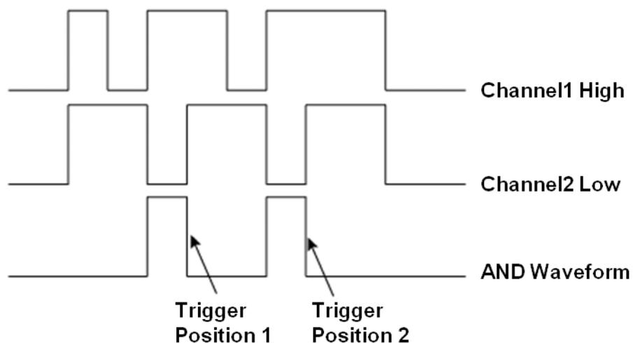
Logic (AND, OR, NAND, NOR), source, limit range, and time value can be set in the trigger dialog box. When the logic is "OR" or "NAND", the setting of the time limit is invalid.
