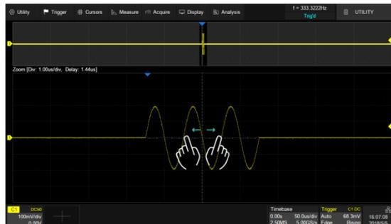
Adjust the horizontal scale of the Zoom window by horizontal pinch and spread in the zoom area of the main window or in the Zoom window
