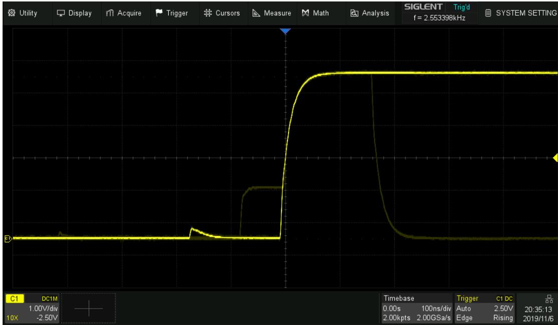
In this case, the zone trigger is a quick and simple way to capture the interesting waveform. Enable the zone trigger, and draw a box to intersect with the bus contention part, as shown in the figure below:
