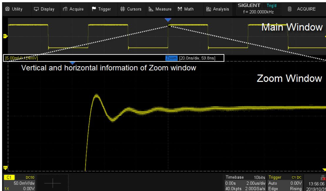
The area not covered by the gray background in the main waveform area is the region to be zoomed in (zoom area). When the zoom window is activated, the zoom area can be expanded or compressed by rotating the horizontal and vertical scale knob. Rotating the horizontal and vertical position knob to move the position of the region. When the main window is activated, the scale knobs and position knobs are used to change the
