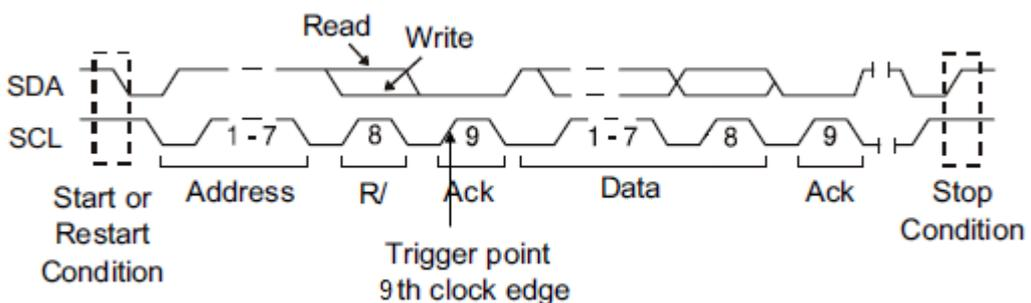
Frame (Start: 7-bit address: R/W: Ack: Data: Ack: Data2)—If all bits match, then trigger on the Ack bit followed by the Data2.
