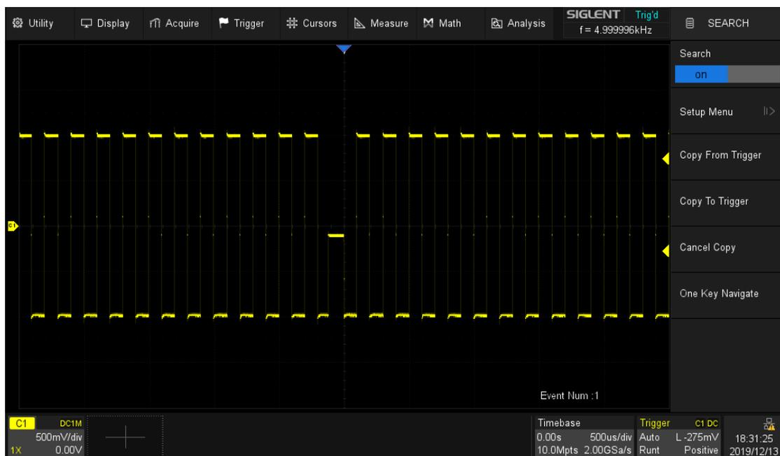
Then turn on the Search function and operate *Copy from Trigger* in the search dialog box so that the oscilloscope searches for the dwarf pulses according to the same setting as the trigger.
