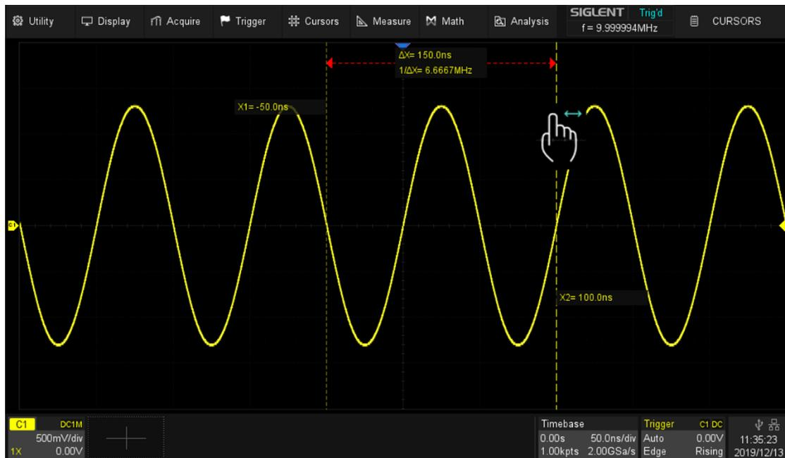
Touch the display area of  $\Delta X$  (or  $\Delta Y$ ) in M1 mode and drag it to move the two cursors simultaneously, as shown in the figure below. This is equivalent to the operation on the cursor type X1-X2 or Y1-Y2.
