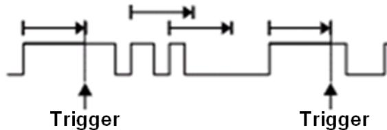
Trigger source, slope (rising, falling), dropout type and time value can be set in the trigger dialog box. Holdoff, coupling, and noise reject can be set in the dropout trigger, see the sections " Holdoff", " Trigger Coupling" and " Noise Reject" for details.
