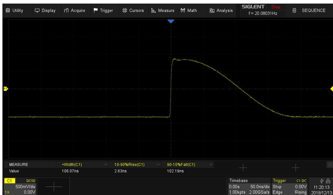
In the example, 5000 pulses can be obtained with the sample rate of 2 GSa/s at the maximum memory depth.
