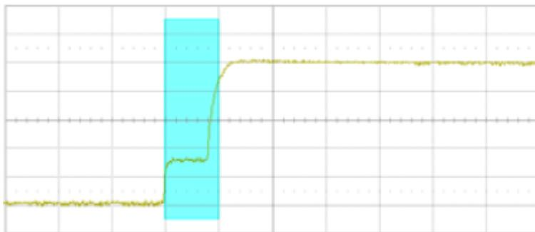
With a simple edge trigger, it is unlikely to trigger consistently on this
