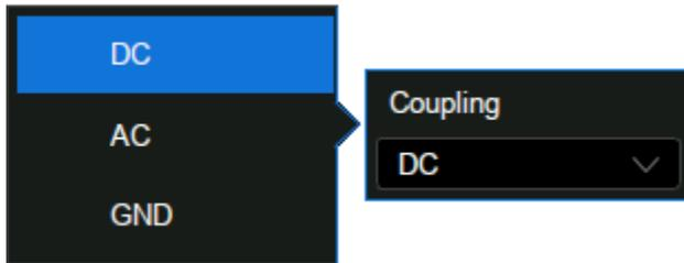
**List:** Sets parameters with more than two options, such as the coupling mode of channels. Touch the parameter region, and then select the expected option from the pop-up list.
