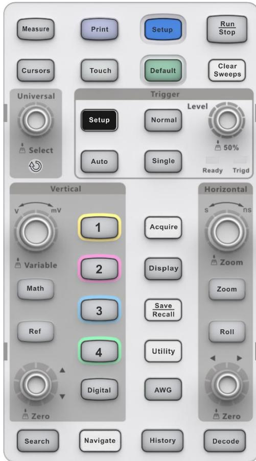
The front panel is designed to operate the basic functions without having to open the software menu. Most of the front panel controls duplicate functionality available through the touch screen display but the operation is more quickly achieved.
