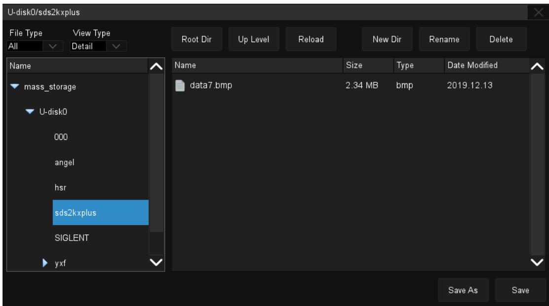
In step 4, if **Save** is selected instead of **Save As**, the system saves the file as the default file name `sds2000X Plus_BMP_n.bmp`, where `n` is an integer incrementing from 1. The default save path is `\SIGLENT\`.
