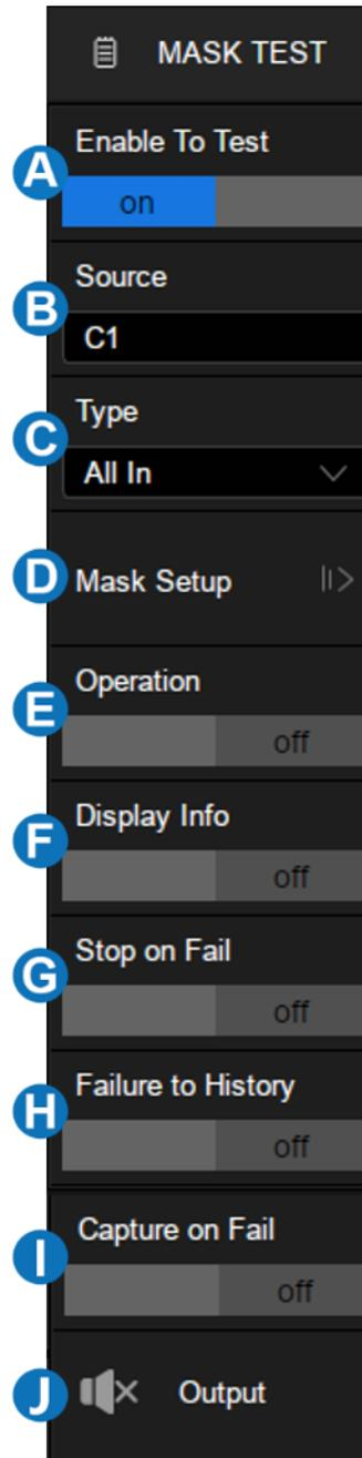
When it is "on", the failure waveform is detected, the screenshot with failure frame will be stored in the external U disk.
