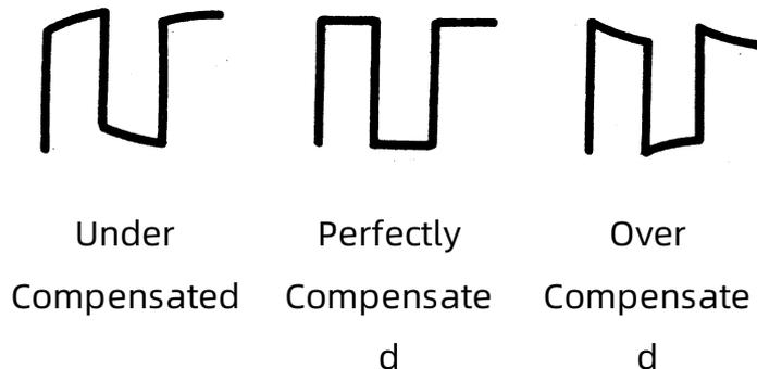
5. Use a non-metallic driver to adjust the low-frequency
