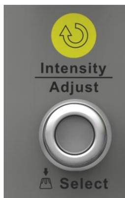
When the parameter setting area is highlighted, you can use the Universal Knob to adjust or set the parameter. Press the knob to select an option from the list. The default function of the Universal Knob is to adjust the intensity of the waveform traces.
