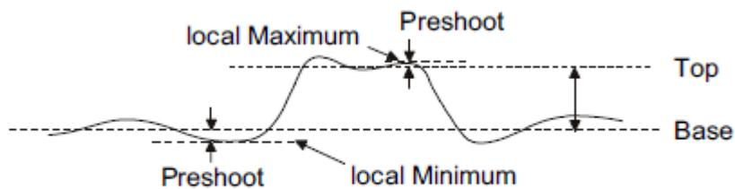
$$\text{Falling Edge Preshoot} = \frac{\text{Maximum} - \text{Top}}{\text{Amplitude}} \times 100\%$$
