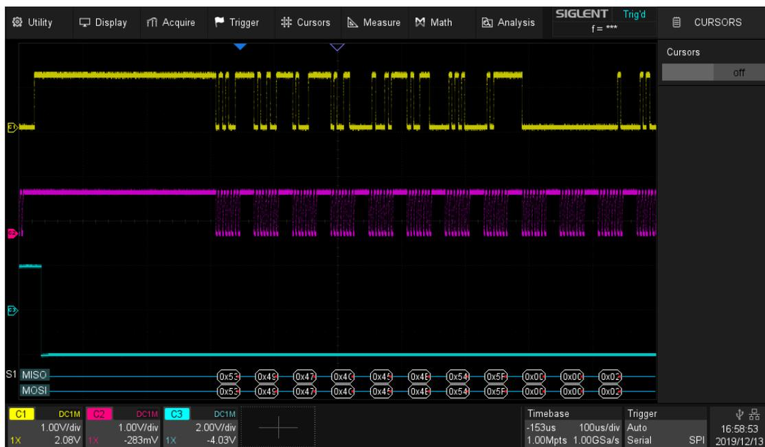
When the CS type is set to Clock Timeout, turn on Cursor, measure the clock idle time between frames as 300  $\mu$ s, and measure the interval between clock pulses as 2.4  $\mu$ s, then set the timeout to a value between 2.4 and 300  $\mu$ s. In this example it is set to 10  $\mu$ s:
