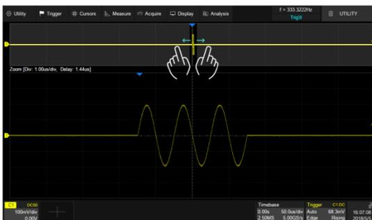
Adjust the horizontal scale of the main window by pinch and spread in the gray area of the main window
