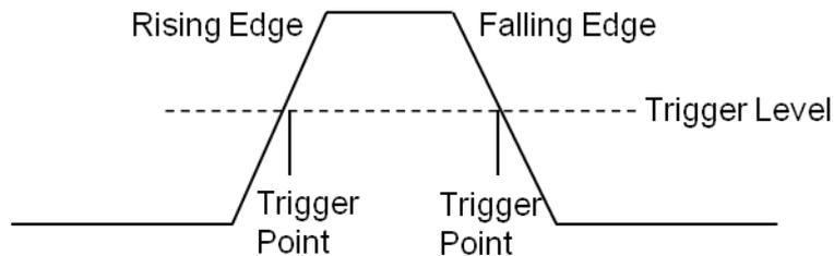
Touch the **Source** area to select trigger source, and touch the **Slope** area to select rising, falling or alter.
