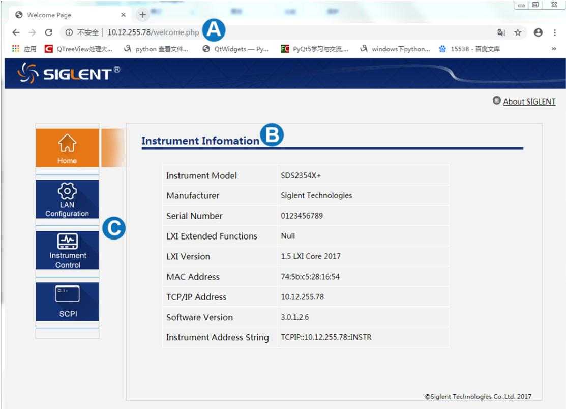
The screenshot shows a web browser window displaying the Siglent instrument's web interface. The browser's address bar shows the IP address 10.12.255.78. The interface includes a navigation menu on the left with options: Home, LAN Configuration, Instrument Control, and SCPI. The main content area is titled "Instrument Information" and contains a table with the following data:
