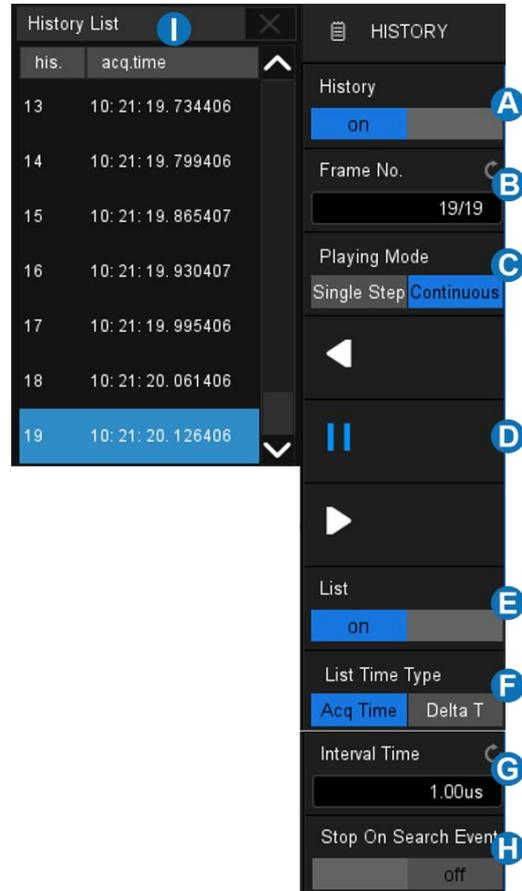
The oscilloscope automatically stores acquired frames. It can store up to 90,000 frames but the number may vary due to the memory depth and timebase settings. Turn on history mode, then the stored frames can be
