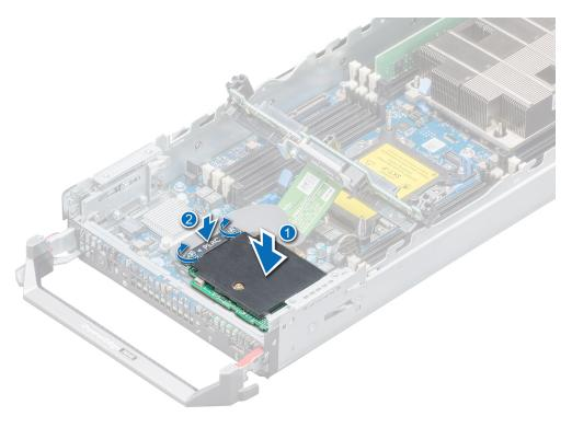
Figure 47. Installing the storage controller card
