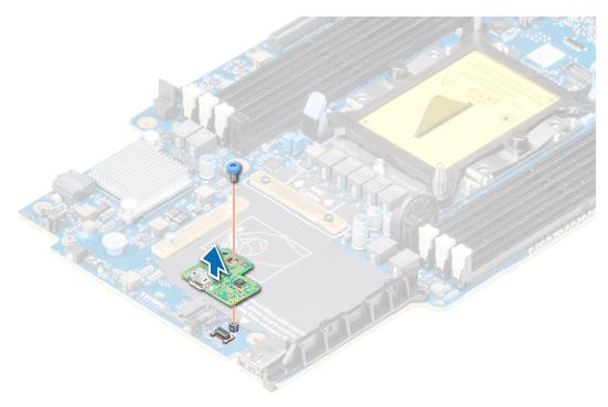
Figure 58. Removing the rSPI card
