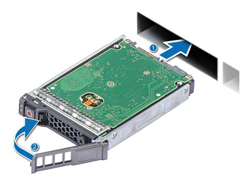
Figure 19. Installing a drive carrier
