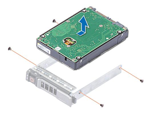
Figure 20. Removing the drive from the drive carrier
