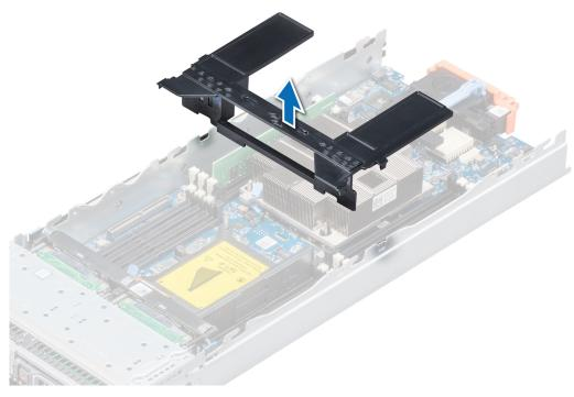
Figure 14. Removing the air shroud
