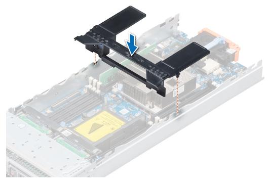
Figure 15. Installing the air shroud
