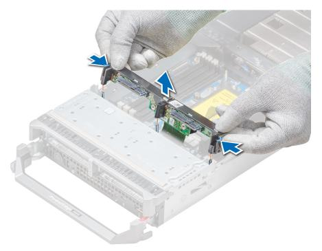
Figure 24. Removing the drive backplane
