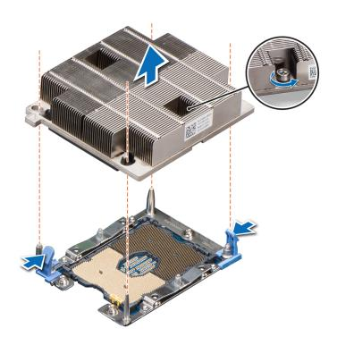
Figure 31. Removing the processor and heat sink module
