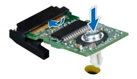
Figure 57. Installing the TPM
