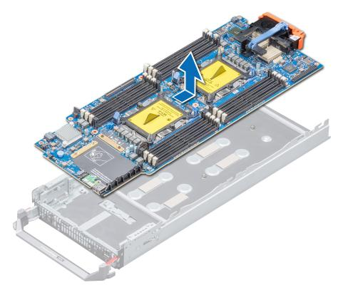
Figure 55. Removing the system board
