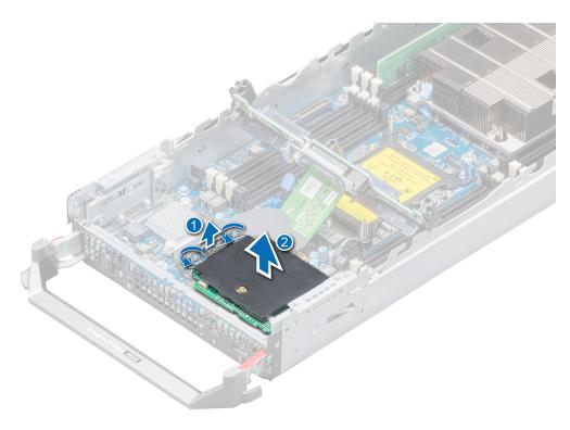
Figure 46. Removing the storage controller card
