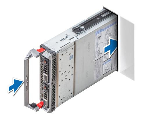
Figure 10. Installing the system into the enclosure
