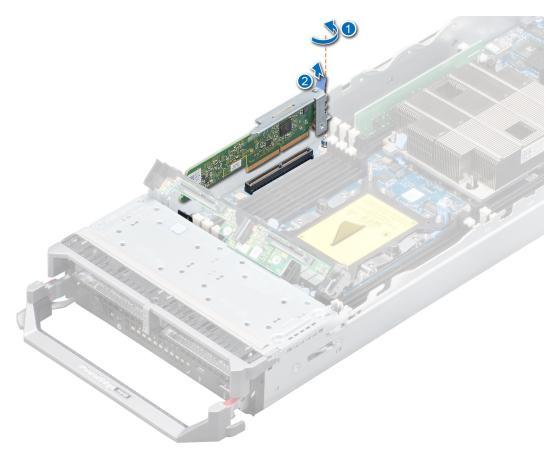
Figure 52. Removing the optional IDSDM module
