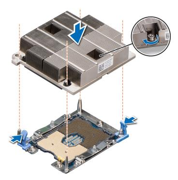
Figure 37. Installing a processor and heat sink module
