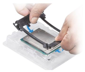
Figure 34. Installing the processor bracket
