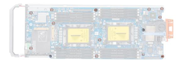
Figure 54. Locations of the screws on the system board
