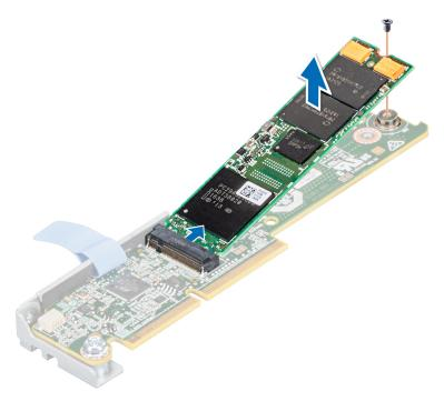
Figure 41. Installing the BOSS card
