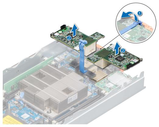
Figure 44. Removing the mezzanine card
