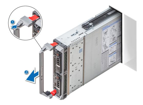
Figure 7. Removing the system from the enclosure
