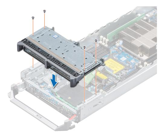
Figure 23. Installing the drive cage
