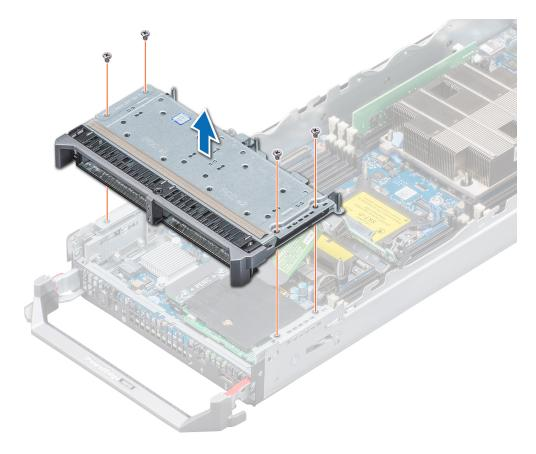
Figure 22. Removing the drive cage
