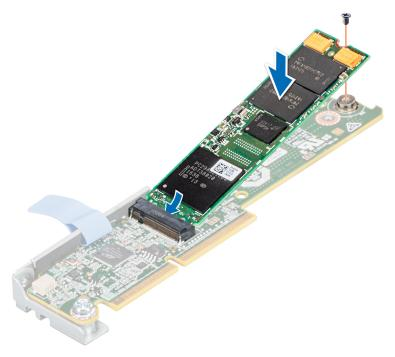
Figure 40. Removing the BOSS card
