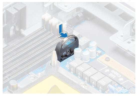
Figure 49. Installing the system battery
