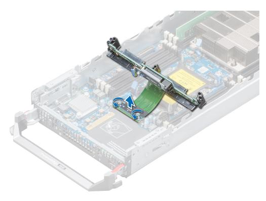
Figure 25. Removing the backplane cable
