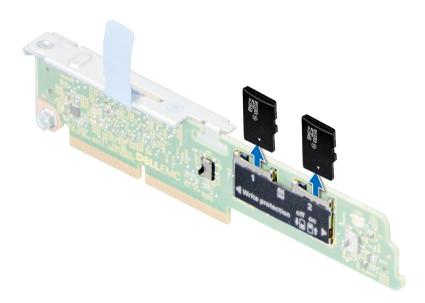
Figure 50. Removing a MicroSD card
