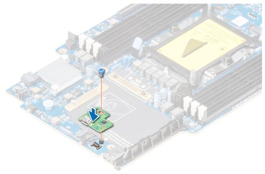
Figure 59. Installing the rSPI card
