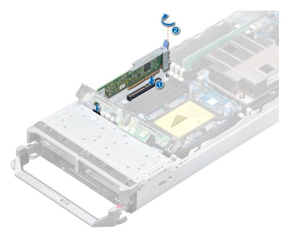
Figure 53. Installing the optional IDSDM module
