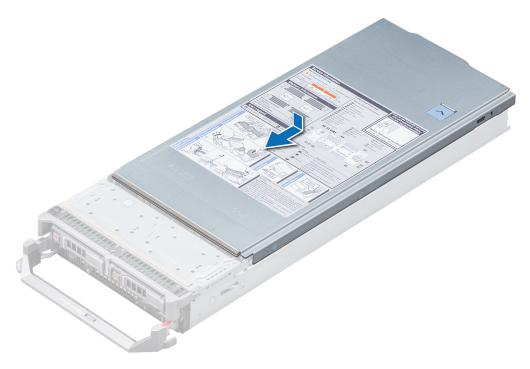
Figure 13. Installing the system cover
