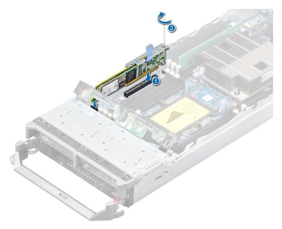
Figure 39. Installing the M.2 BOSS module
