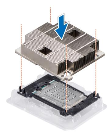
Figure 36. Installing the heat sink onto the processor
