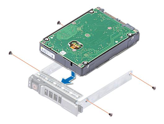
Figure 21. Installing a drive into the drive carrier
