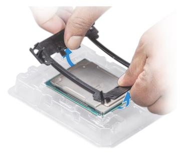
Figure 33. Removing the processor bracket
