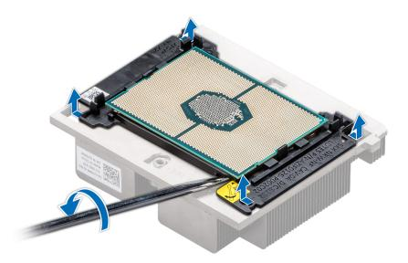
Figure 32. Loosening the processor bracket
