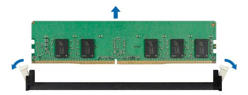
Figure 29. Removing a memory module
