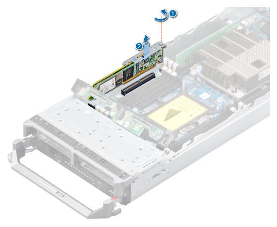
Figure 38. Removing the M.2 BOSS module
