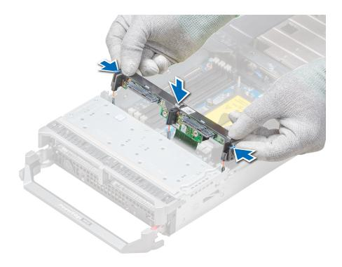
Figure 27. Installing the drive backplane
