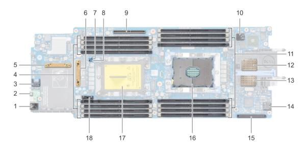
Figure 60. System board connectors
