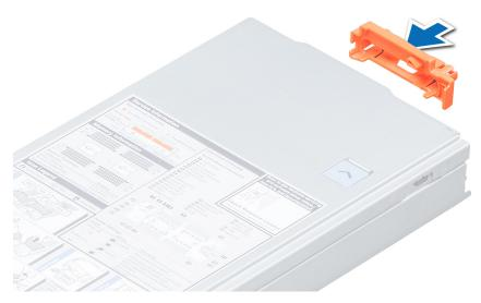
Figure 8. Installing the I/O connector cover
