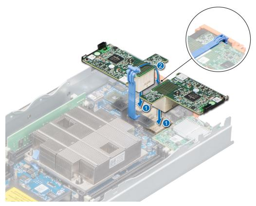
Figure 45. Installing the mezzanine card
