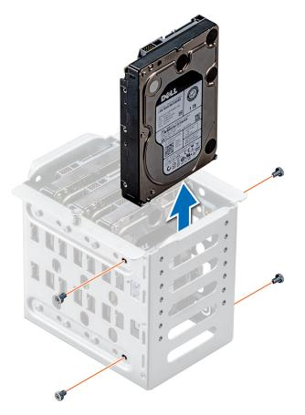
Figure 43. Removing a cabled drive
