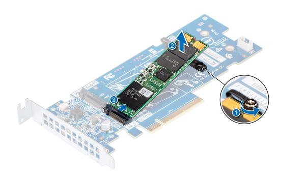
Figure 66. Removing the M.2 SSD module
