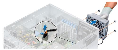
Figure 58. Removing the external cooling fan
