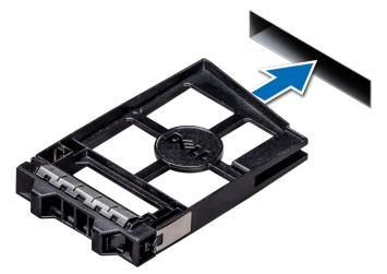
Figure 28. Installing a drive blank
