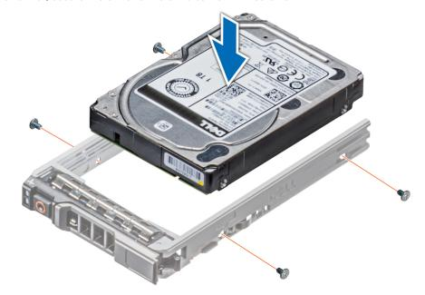
Figure 32. Installing a drive into the drive carrier
