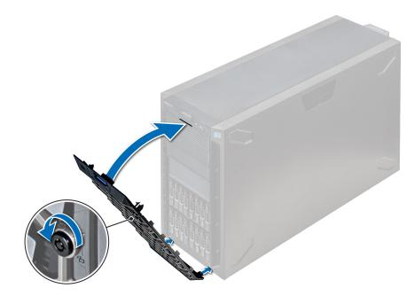
Figure 16. Installing the front bezel
