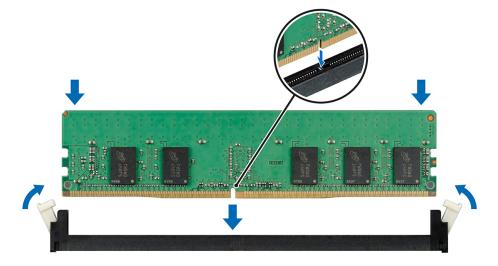
Figure 55. Installing a memory module
