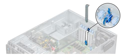
Figure 64. Removing the filler bracket
