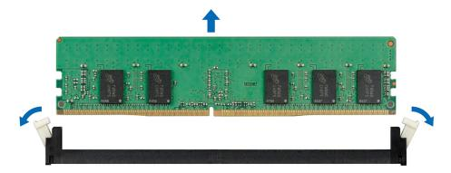
Figure 54. Removing a memory module
