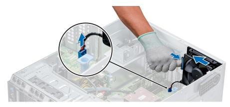
Figure 56. Removing the internal cooling fan
