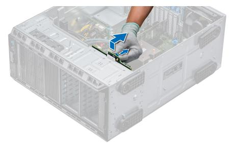
Figure 51. Removing a backplane
