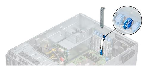
Figure 63. Installing the filler bracket
