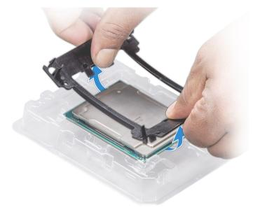
Figure 74. Removing the processor bracket
