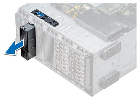
Figure 37. Removing the optical drive or tape drive blank
