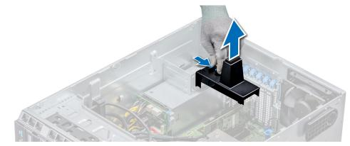
Figure 60. Removing the expansion card holder
