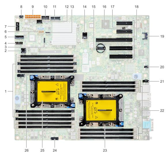
Figure 97. T440 system board jumpers and connectors
