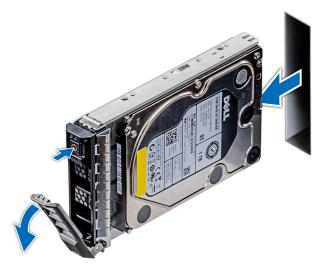
Figure 29. Removing a drive carrier
