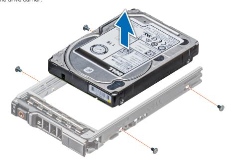
Figure 31. Removing the drive from the drive carrier
