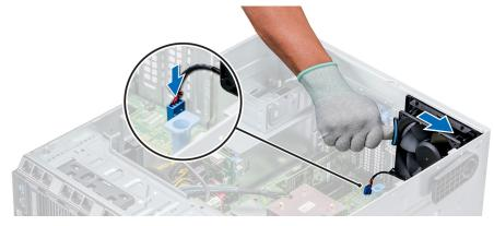
Figure 57. Installing the internal cooling fan
