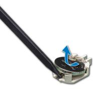
Figure 87. Removing the system battery
