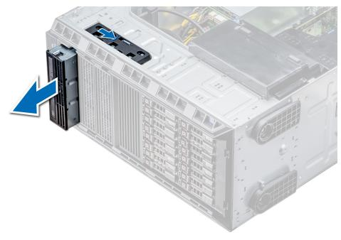
Figure 39. Removing the optical drive cage or tape drive
