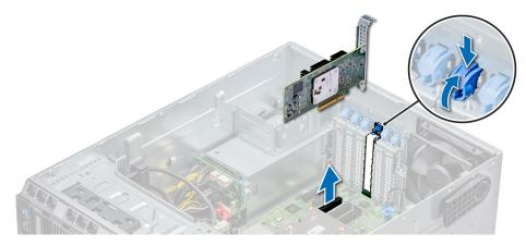
Figure 62. Removing an expansion card
