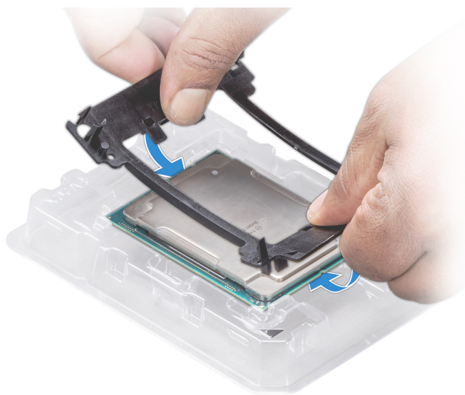
Figure 60. Installing the processor bracket
