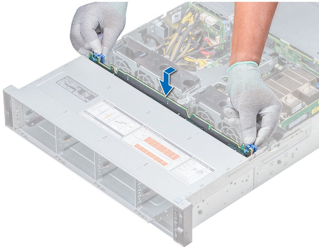
Figure 101. Installing the backplane
