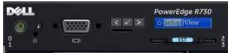
Figure 9. R730 LCD control panel
