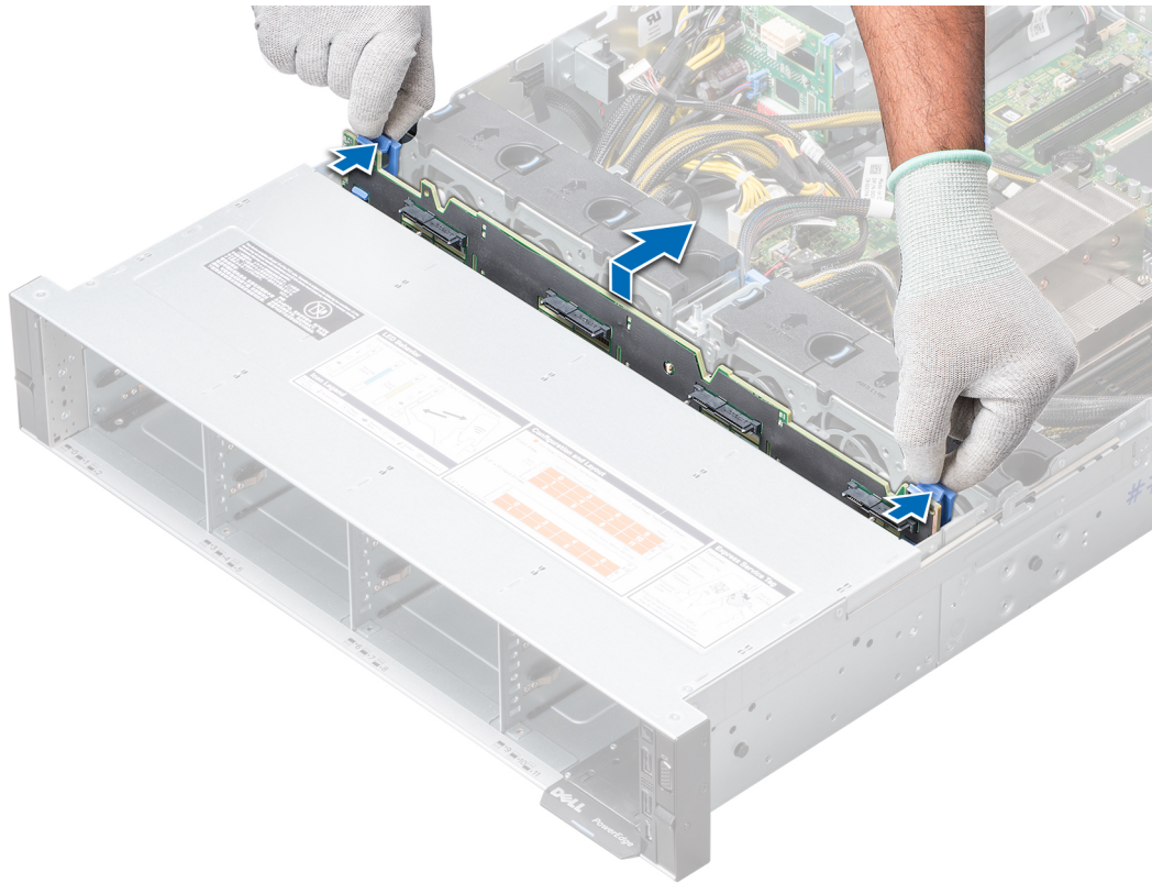
Figure 64. Removing the drive backplane
