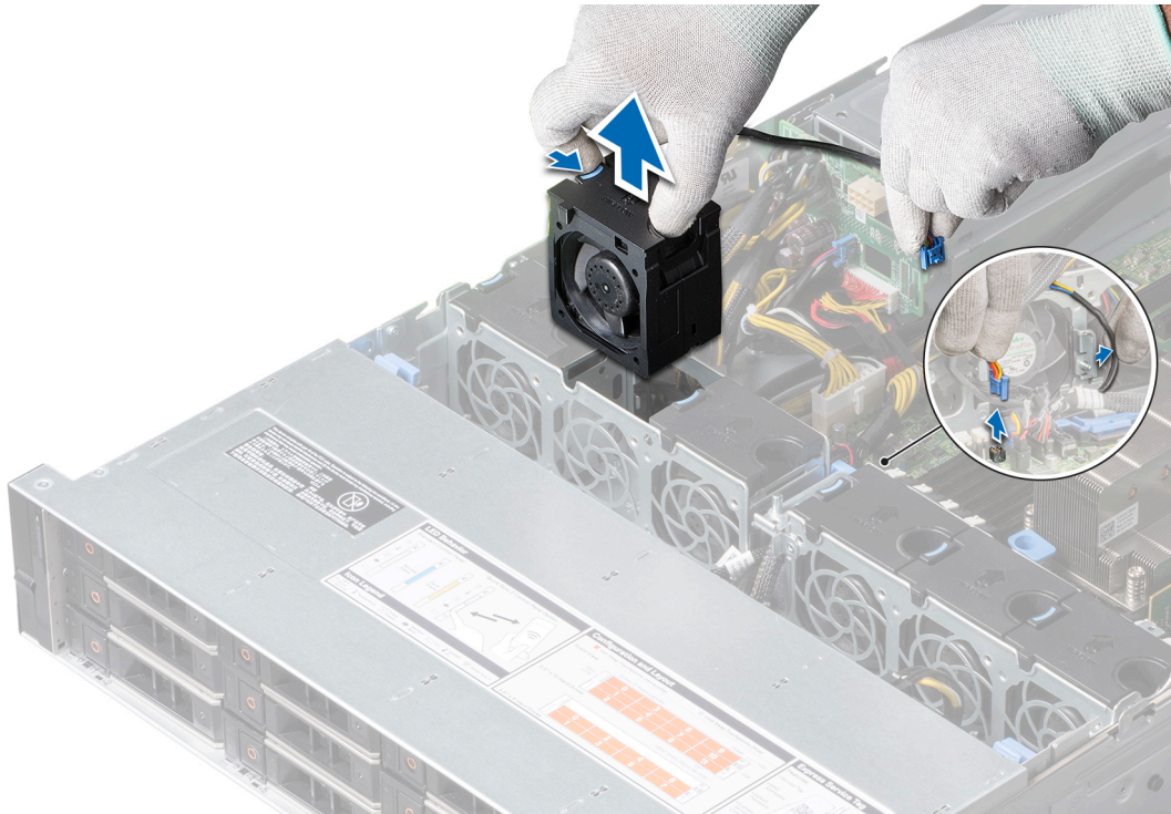
Figure 34. Removing a cooling fan
