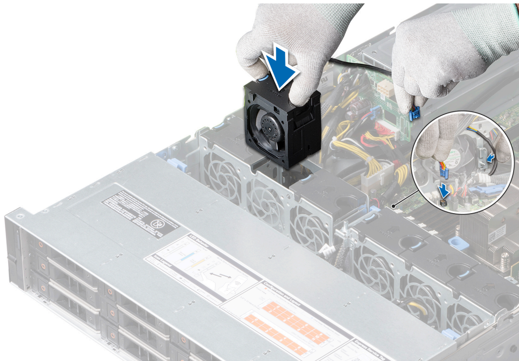
Figure 36. Installing a cooling fan
