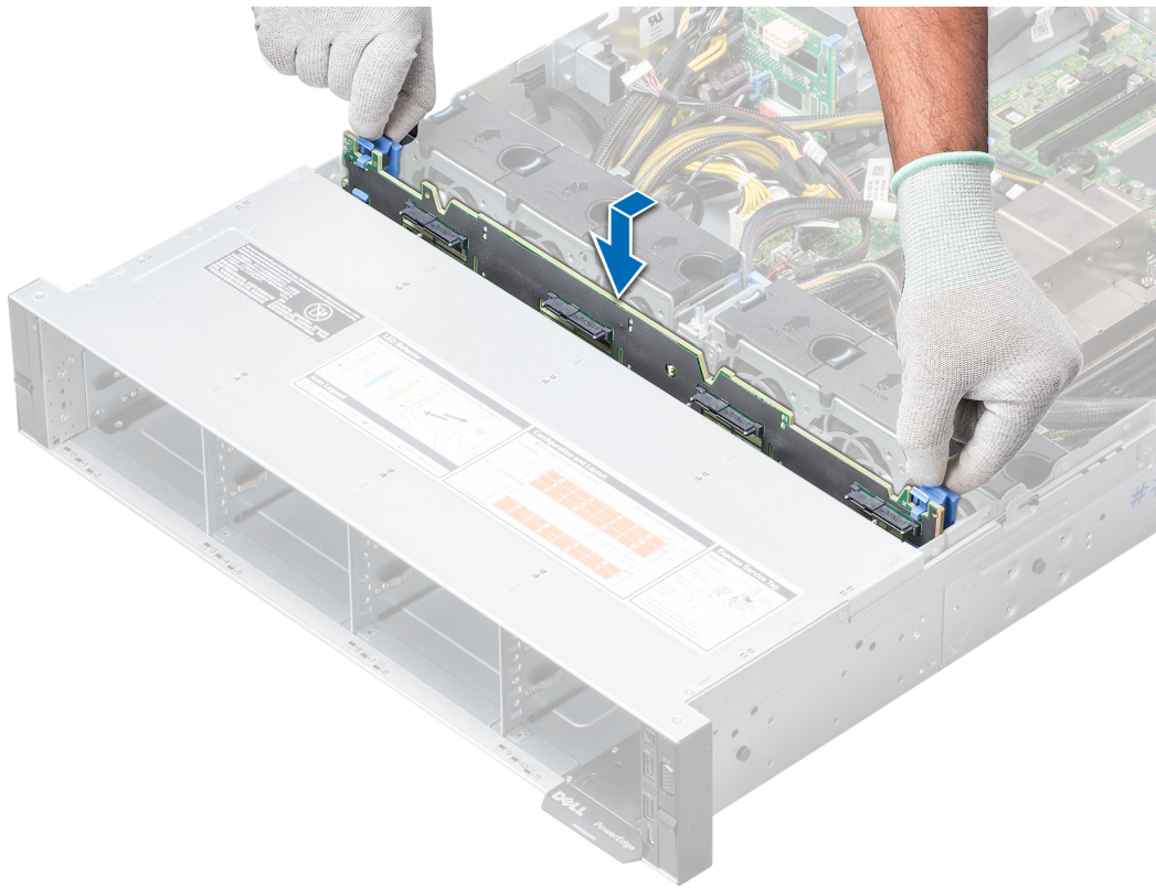
Figure 65. Installing the drive backplane
