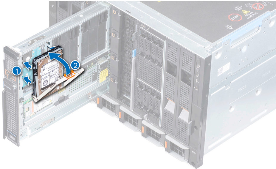
Figure 16. Installing a drive carrier
