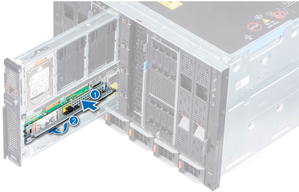
Figure 21. Installing an expander module
