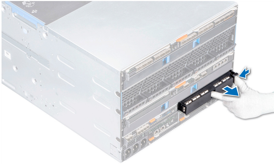
Figure 22. Removing a blank from Fabric C slot
