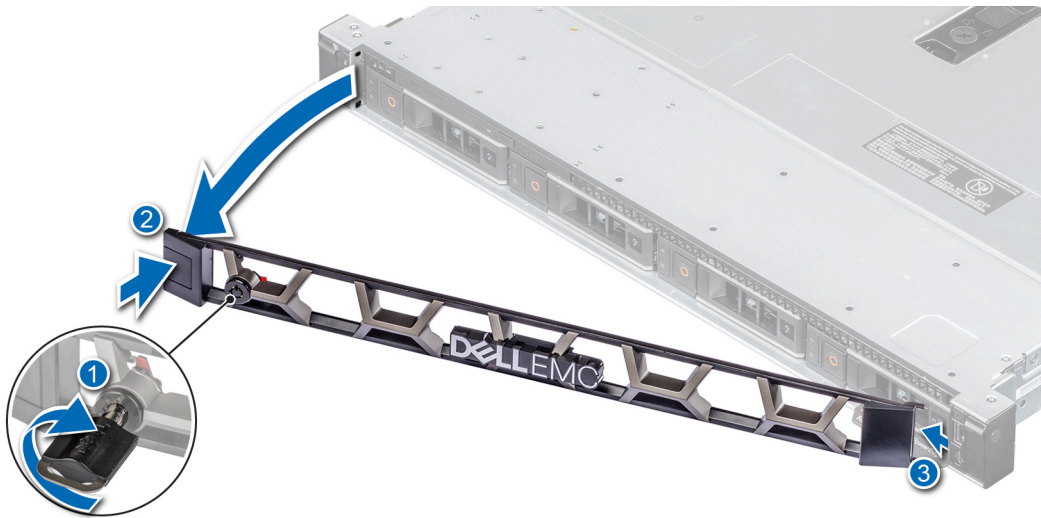
Figure 9. Removing the front bezel
