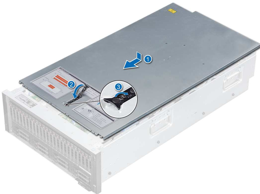
Figure 28. Installing system cover
