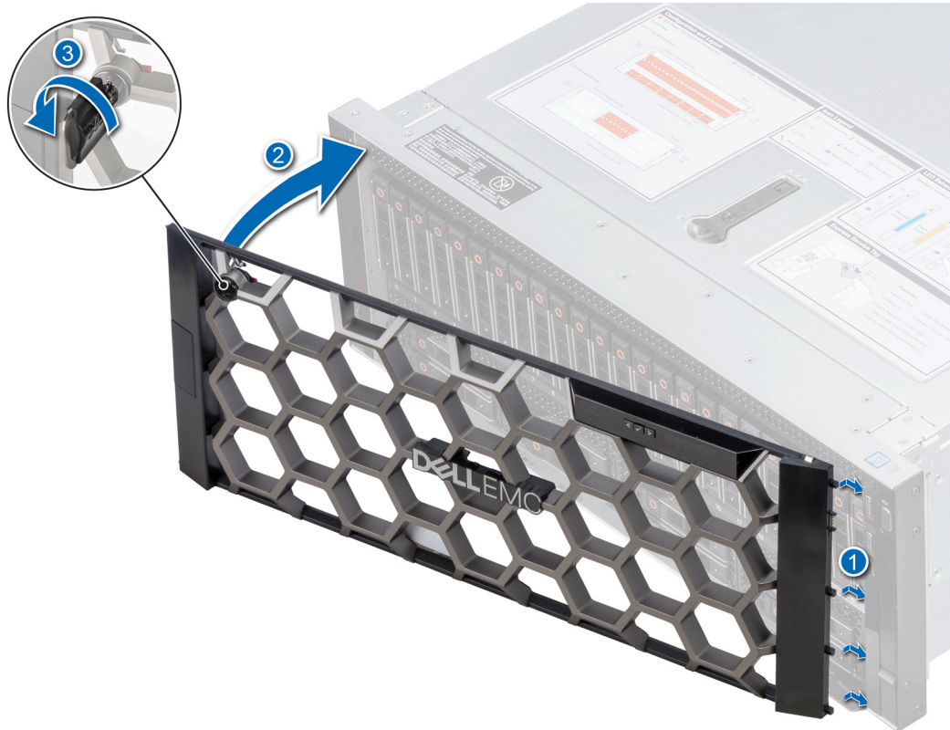
Figure 20. Installing the optional front bezel with the LCD panel
