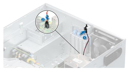
Figure 27. Installing the intrusion switch
