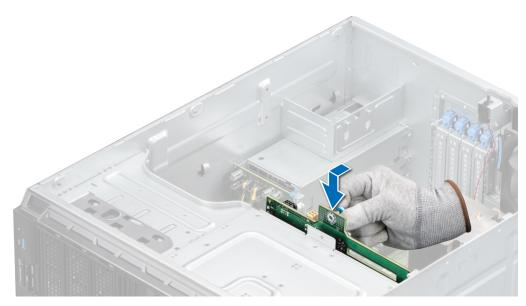
Figure 46. Installing the drive backplane
