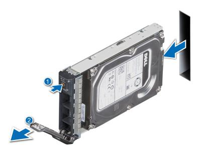
Figure 30. Removing a drive carrier
