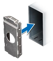
Figure 71. Installing the power supply unit blank
