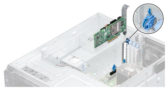
Figure 56. Removing an expansion card
