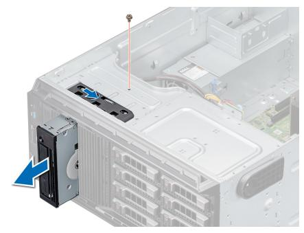
Figure 42. Removing the tape drive
