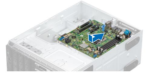
Figure 82. Installing the system board
