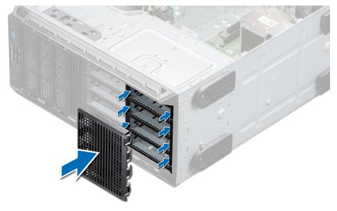
Figure 50. Installing a four-slot drive blank
