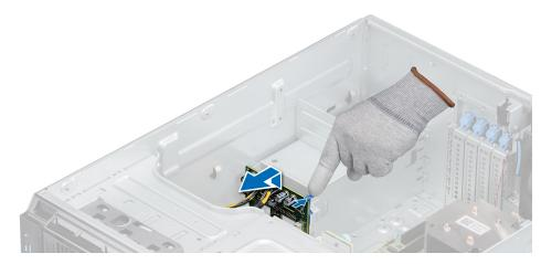
Figure 76. Removing the power interposer board
