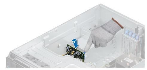
Figure 77. Installing the power interposer board
