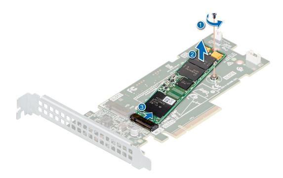
Figure 60. Removing the M.2 SSD module
