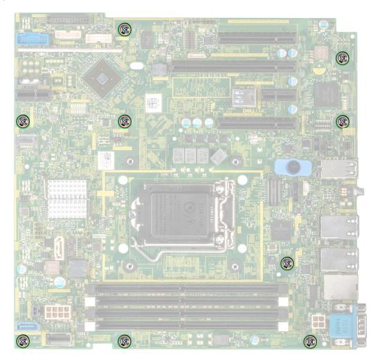
Figure 80. Removing the screws from the system board
