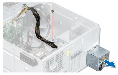
Figure 74. Removing a cabled power supply unit
