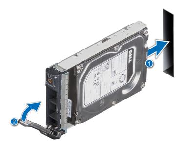
Figure 31. Installing a drive carrier
