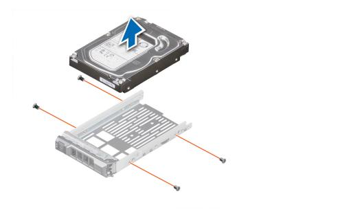
Figure 32. Removing the drive from the drive carrier
