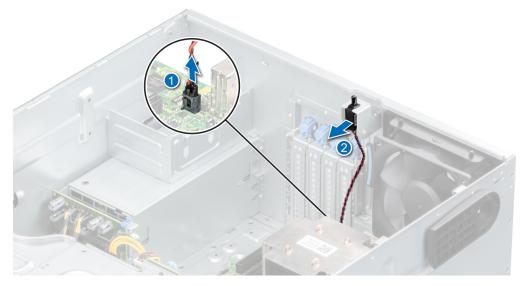
Figure 26. Removing the intrusion switch
