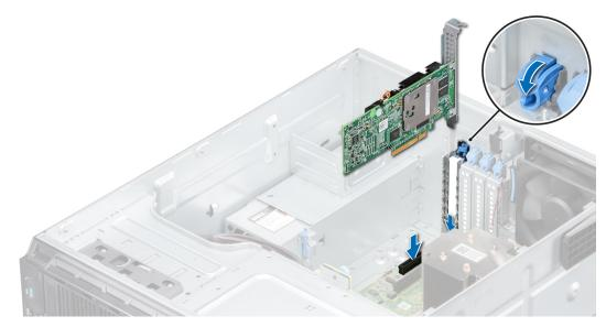
Figure 58. Installing an expansion card
