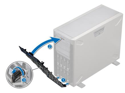
Figure 18. Installing the front bezel
