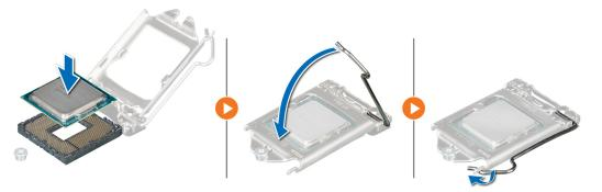
Figure 67. Installing the processor
