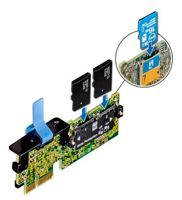
Figure 64. Installing the MicroSD card
