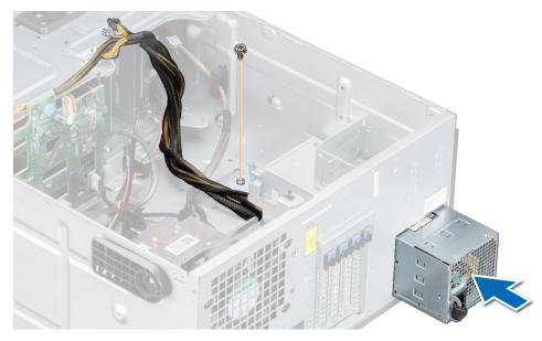
Figure 75. Installing a cabled power supply unit
