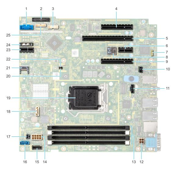
Figure 86. T340 system board jumpers and connectors
