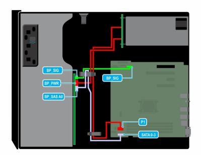
Figure 47. Cable routing - 8 x 3.5-inch, SATA drive backplane
