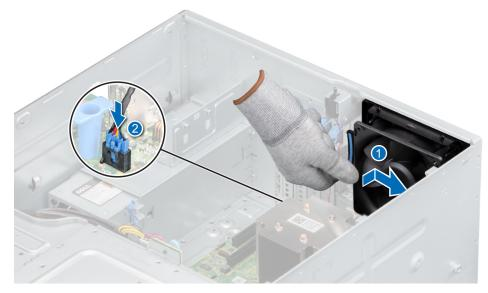
Figure 55. Installing the internal cooling fan
