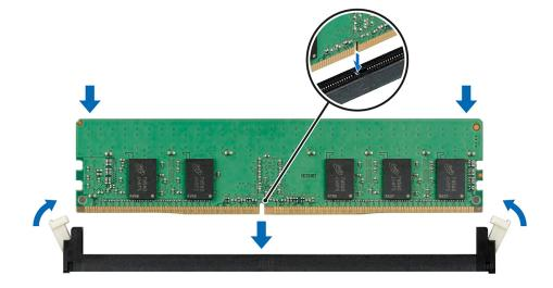
Figure 53. Installing a memory module
