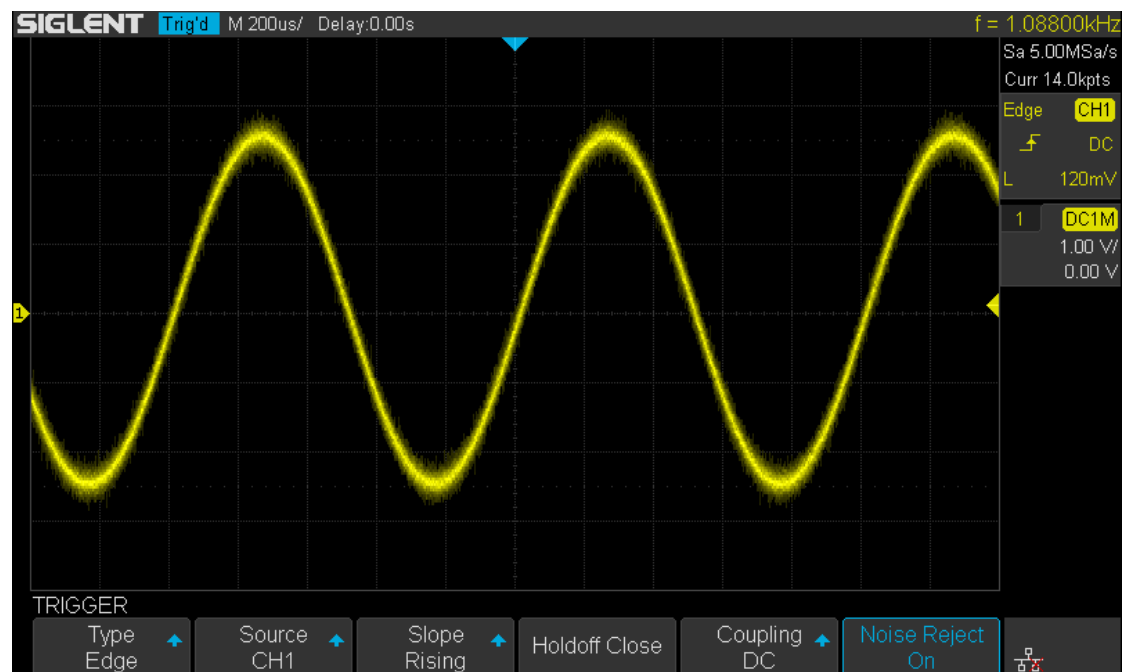
Figure 29 Turn on the Noise Reject
