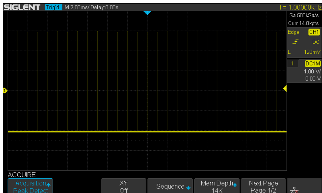
Figure 23 Pulse With 0.1% Duty, Peak Detect Mode
