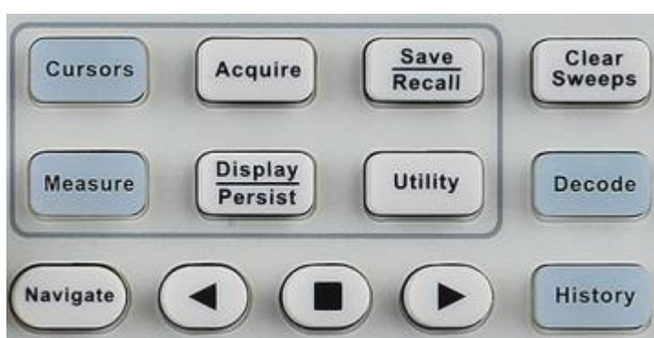
4-channel scope common function panel
