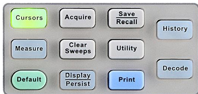
2-channel scope common function panel
