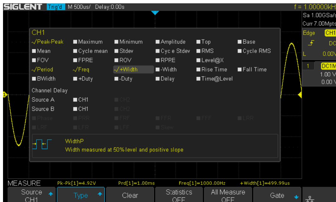
Figure 90 Select the Measurement Parameter
