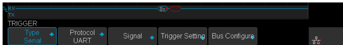
Figure 58 UART Decode Bus Display
