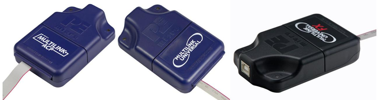
PEmicro's Multilinks allow the user can take advantage of the background debug mode to halt normal processor execution and use a PC to control the processor. The user can then directly control the target's execution, read/write registers and memory values, debug code on the processor, and program internal or external FLASH memory devices. The USB Multilink FX can also provide power to your target MCU, either 3.3V or 5V.
