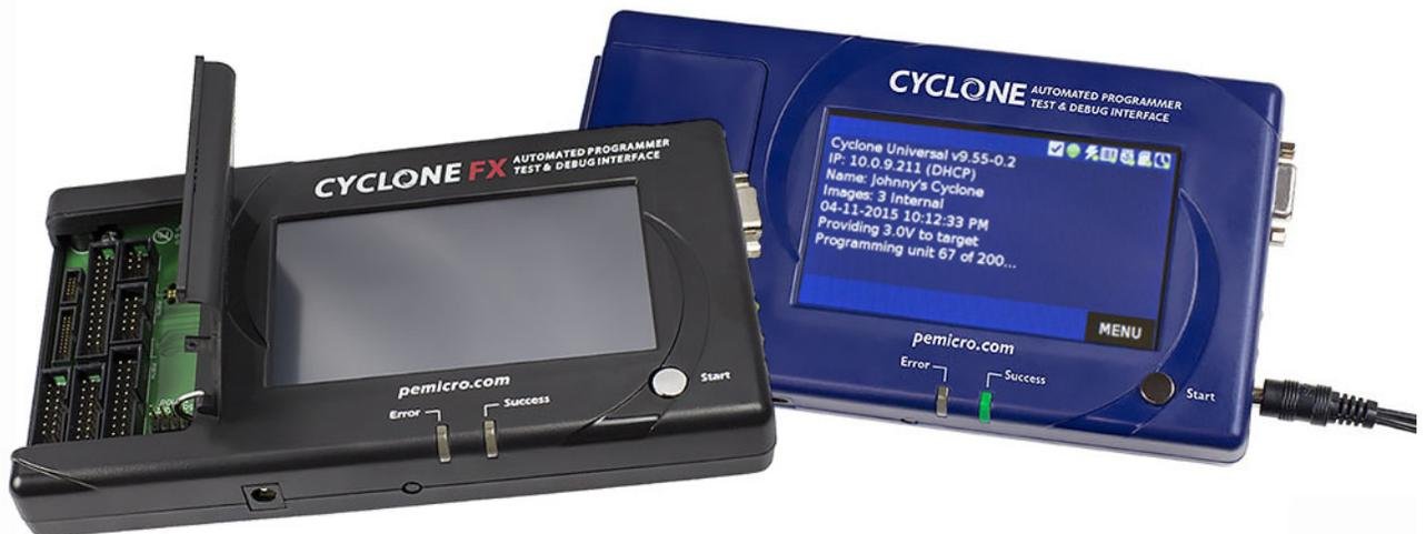
By connecting to a debug header on the target, Cyclone programmers can program internal memory on an ARM Cortex-M processor. SWD/JTAG protocol is used for programming, which requires only 2 pins. The processor or memory device can be mounted on the final printed circuit board before programming.
