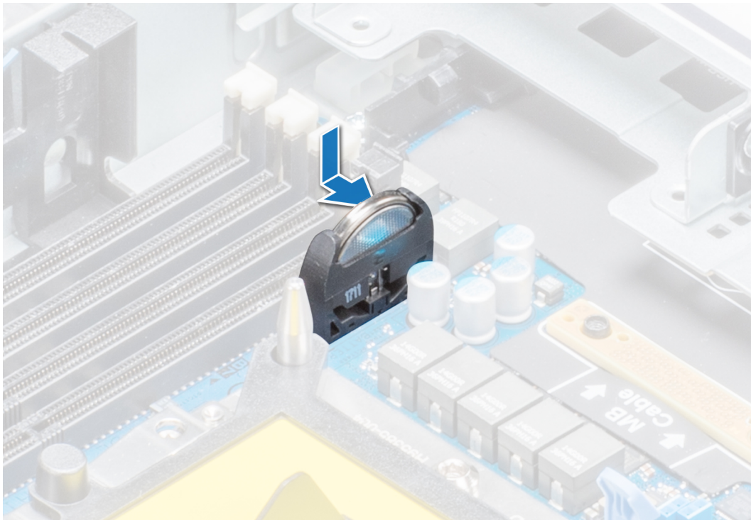
Figure 49. Installing the system battery
