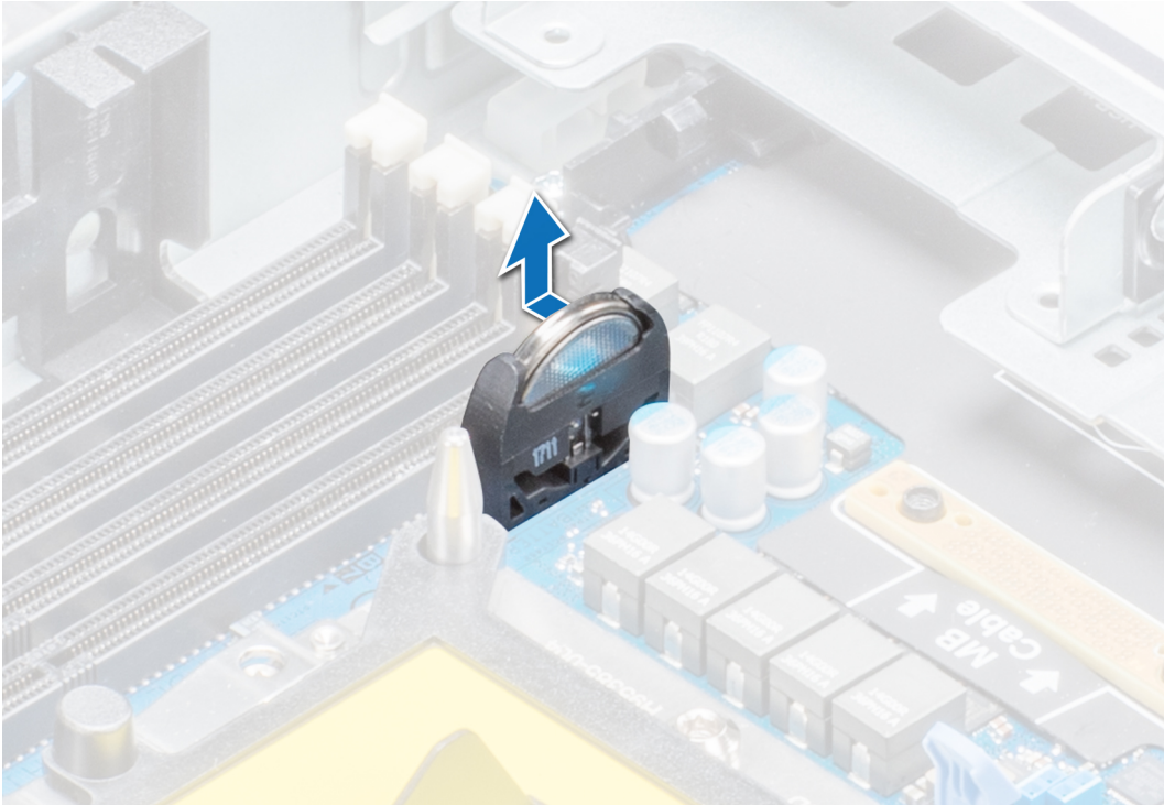
Figure 48. Removing the system battery
