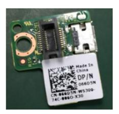
Figure 7. USB Micro-AB with rSPI card
