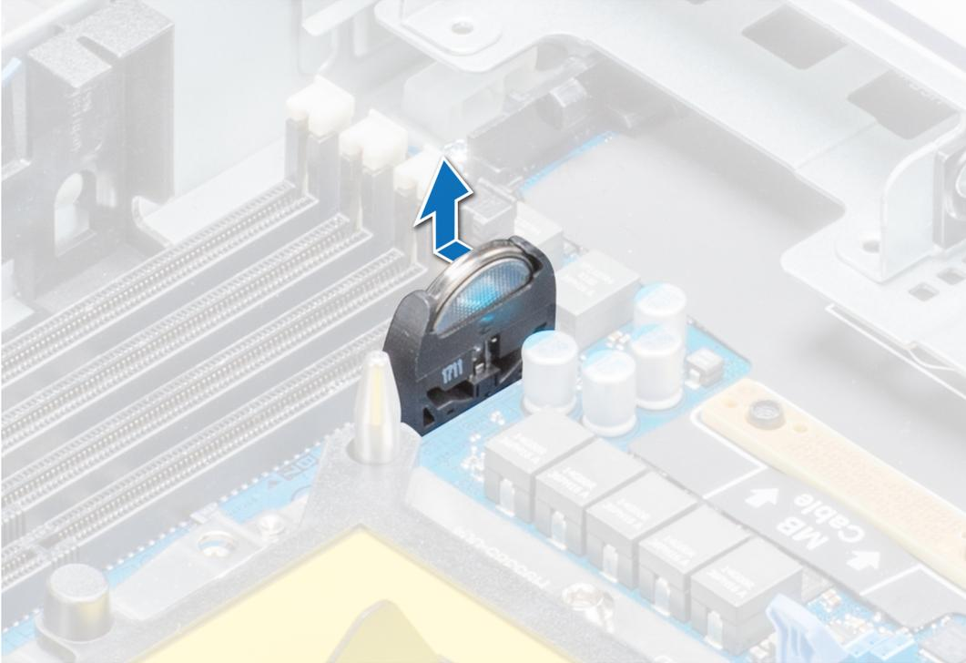
**Figure 48. Removing the system battery**
