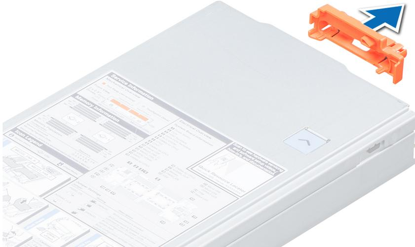
**Figure 9. Removing the I/O connector cover**
