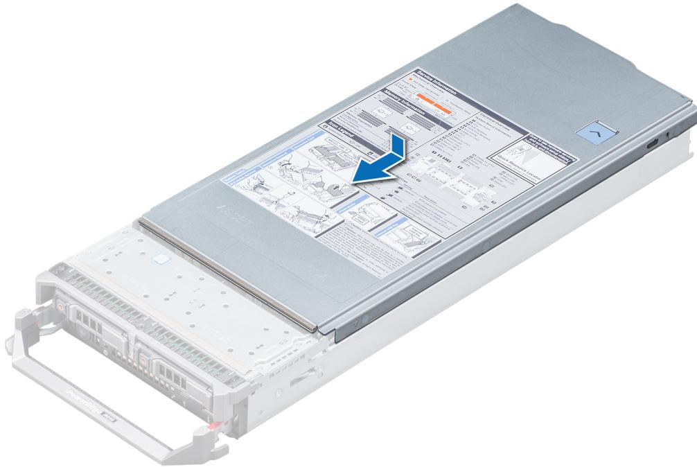
**Figure 13. Installing the system cover**
