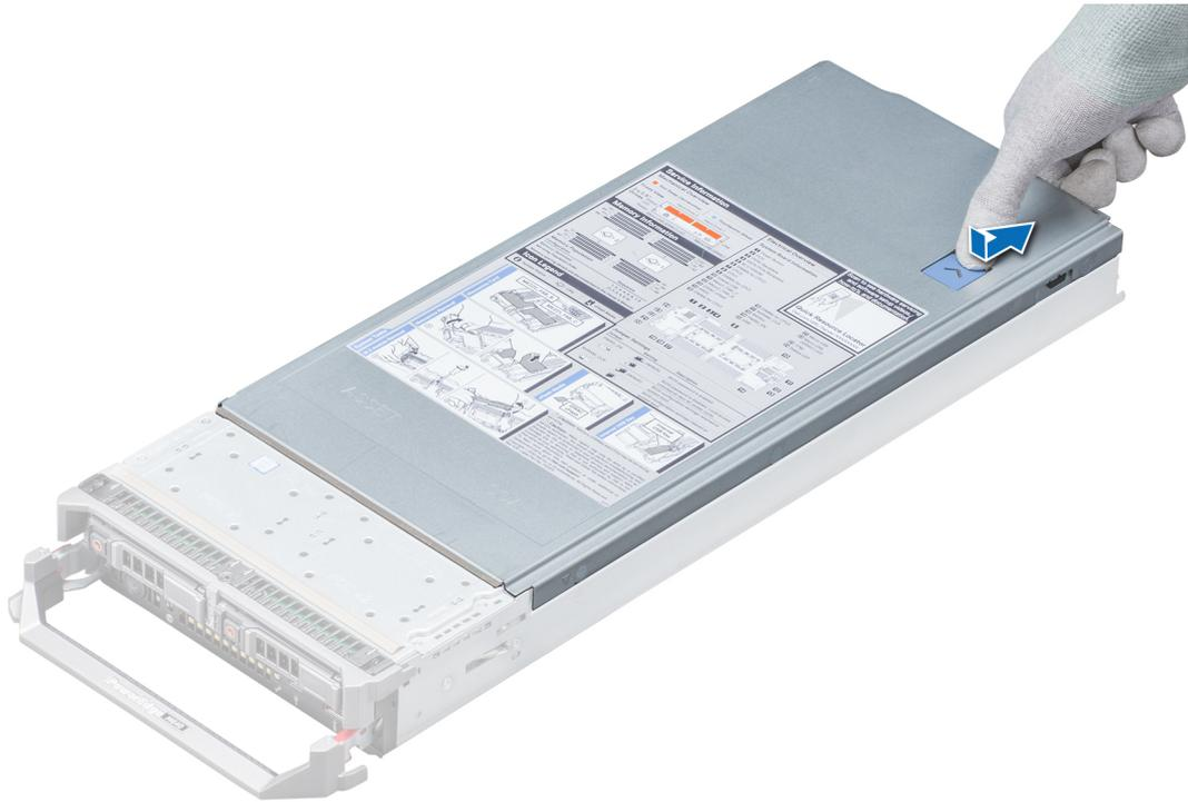
Figure 12. Removing the system cover
