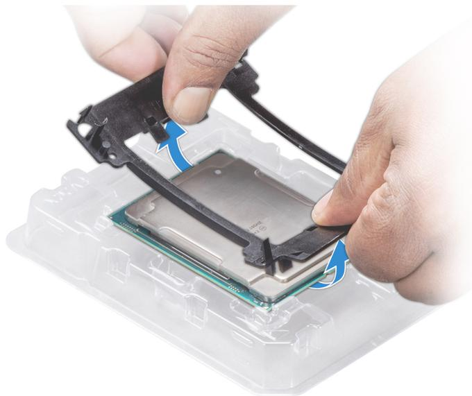
**Figure 33. Removing the processor bracket**
