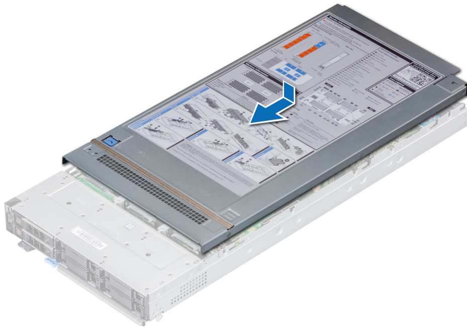
Figure 17. Installing system cover
