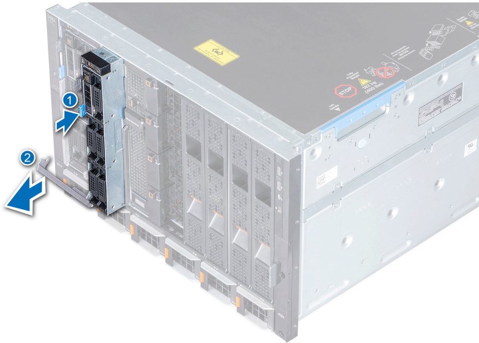
Figure 12. Removing the sled from enclosure
