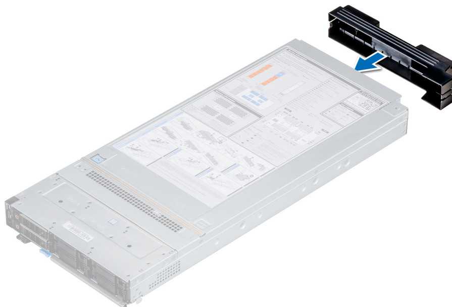
Figure 13. Installing the I/O connector cover on sled
