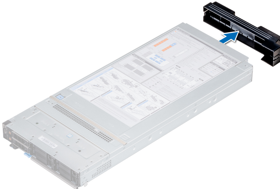
Figure 14. Removing the I/O connector cover from sled
