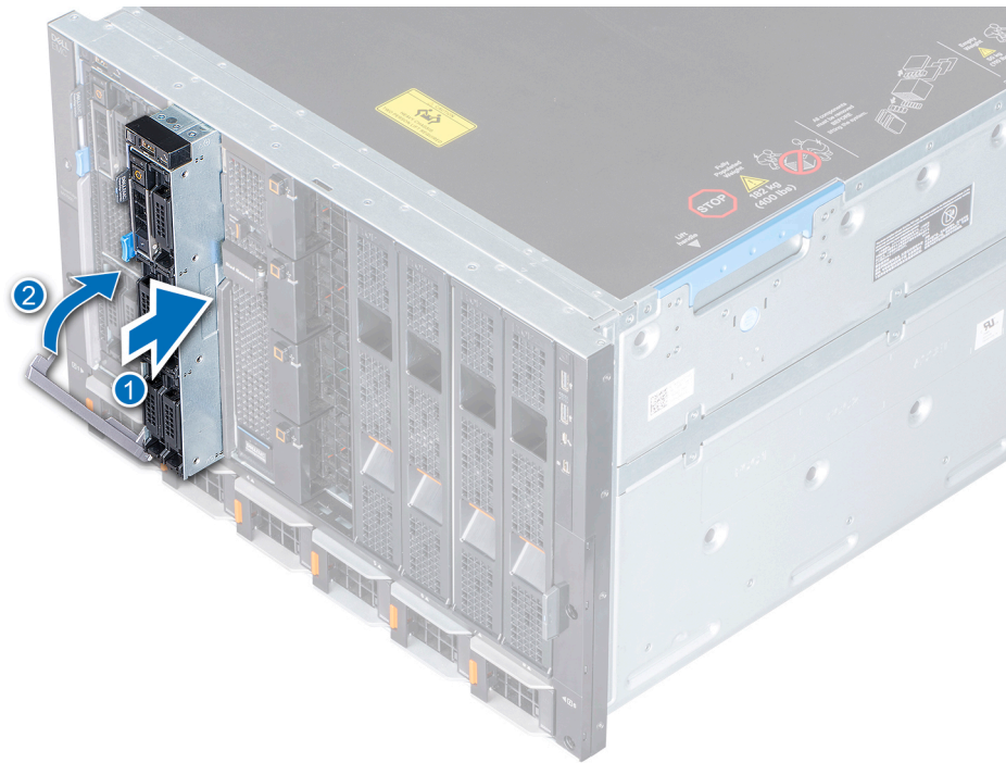
Figure 15. Installing the sled into enclosure
