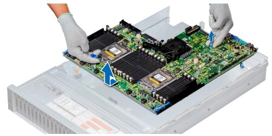
Figure 161. Removing the system board
