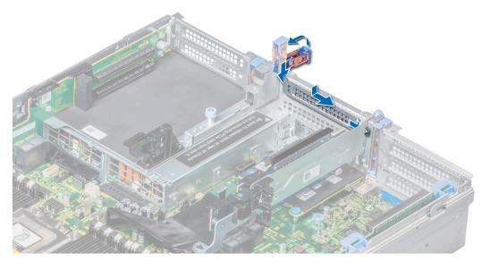
Figure 84. Installing a filler bracket for riser 2
