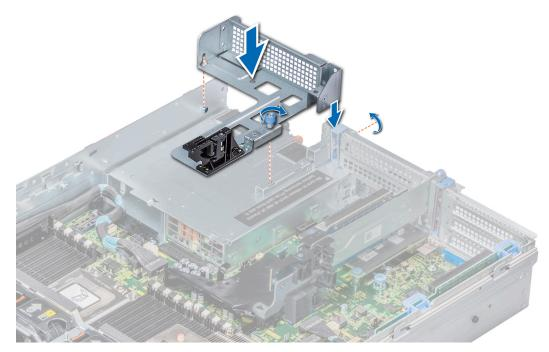
Figure 95. Installing the riser 3 blank
