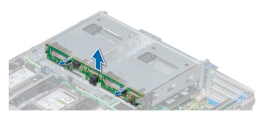
Figure 131. Removing the 3.5 inch rear drive backplane
