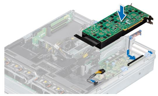
Figure 110. Installing GPU 1
