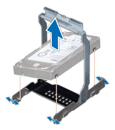
Figure 47. Removing a 3.5 inch drive from the 3.5 inch drive carrier
