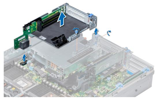
Figure 102. Removing the expansion card riser 3
