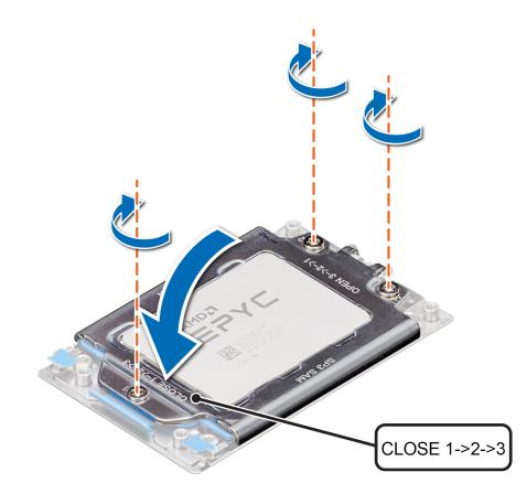
Figure 76. Securing the processor socket cover
