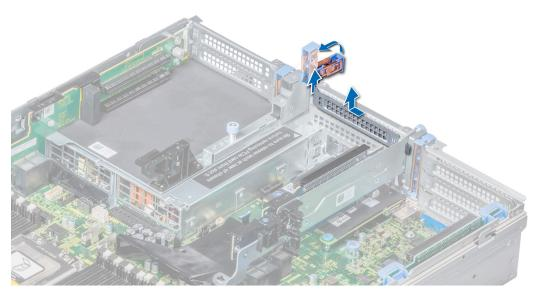
Figure 87. Removing a filler bracket for riser 2
