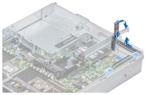
Figure 86. Removing a filler bracket for riser 1
