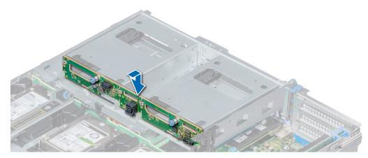
Figure 132. Installing the 3.5 inch rear drive backplane
