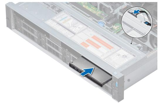
Figure 152. Installing the optional optical drive
