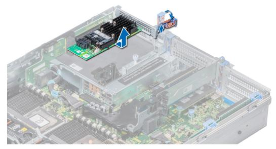
Figure 82. Removing expansion card from expansion card riser 3
