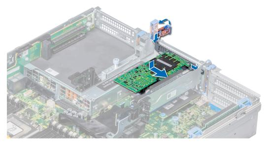
Figure 90. Installing expansion card into the expansion card riser 2
