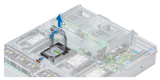
Figure 45. Removing the drive carrier from the mid drive tray
