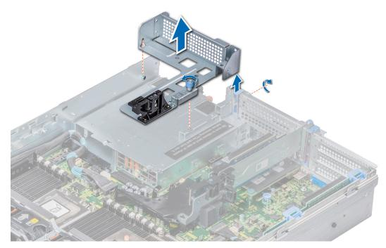
Figure 94. Removing the riser 3 blank
