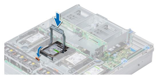
Figure 46. Installing the drive carrier into mid drive tray
