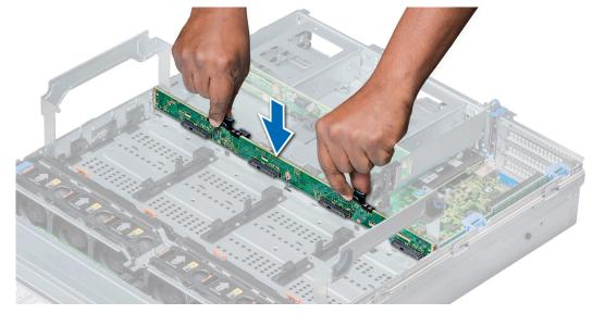
Figure 130. Installing the mid drive tray backplane
