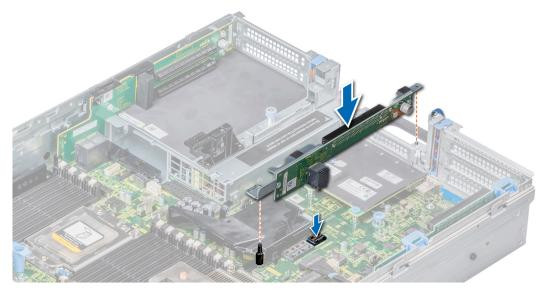
Figure 101. Installing the expansion card riser 2B or 2C
