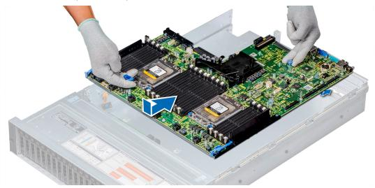
Figure 162. Installing the system board
