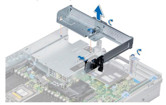
Figure 92. Removing the riser 2 and 3 blank
