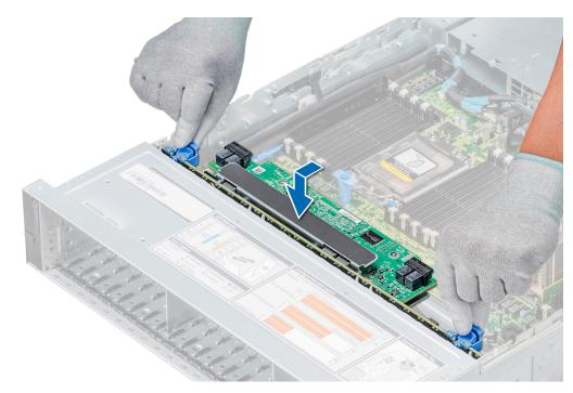
Figure 128. Installing the drive backplane
