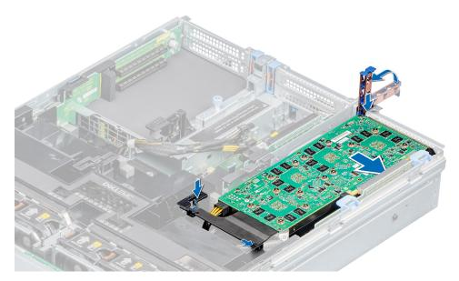
Figure 111. Securing GPU 1
