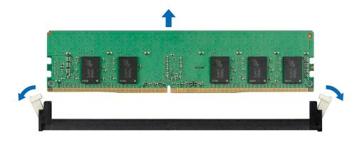
Figure 66. Removing a memory module
