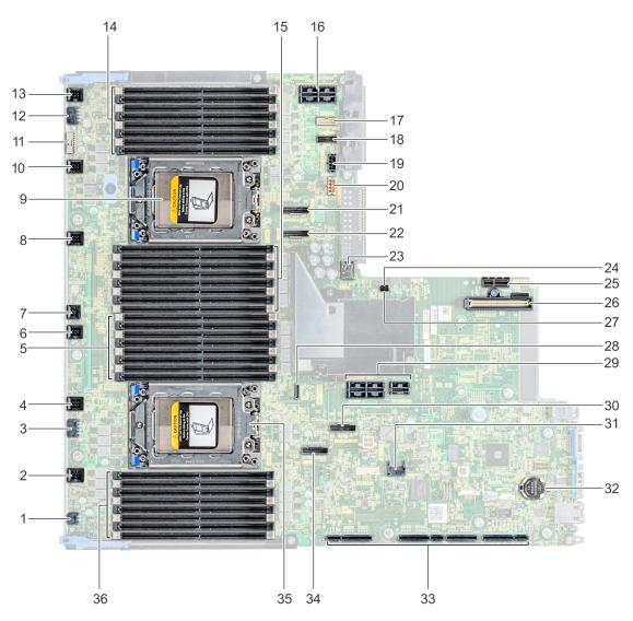
Figure 164. System board jumpers and connectors
