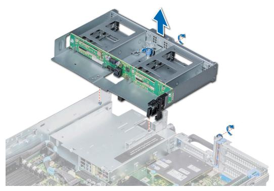
Figure 61. Removing a 4 x 2.5 inch rear hard drive cage
