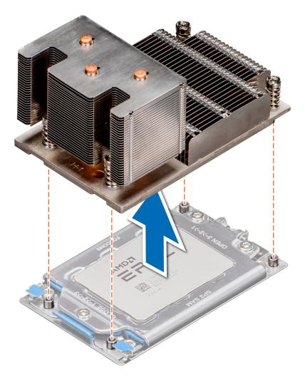
Figure 68. Removing a heat sink
