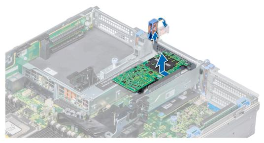
Figure 81. Removing expansion card from expansion card riser 2
