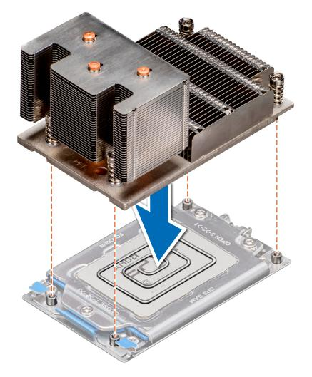
Figure 77. Installing the heat sink
