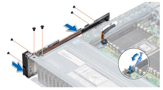
Figure 158. Installing the left control panel
