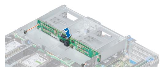
Figure 134. Installing the 2.5 inch rear drive backplane
