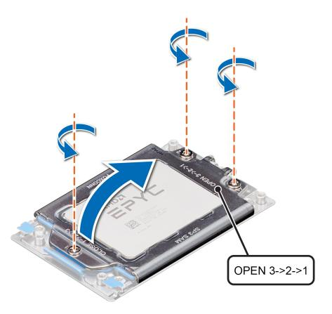
Figure 69. Removing screws on the force plate
