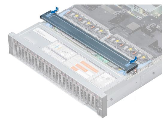
Figure 30. Installing the backplane cover
