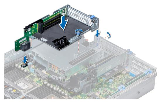
Figure 103. Installing the expansion card riser 3
