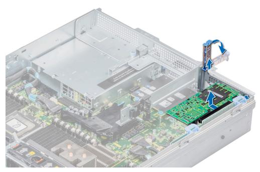
Figure 80. Removing expansion card from expansion card riser 1
