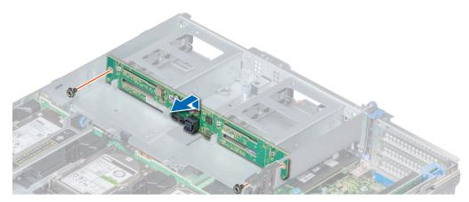
Figure 133. Removing the 2.5 inch rear drive backplane
