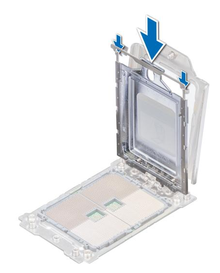
Figure 72. Installing a processor blank
