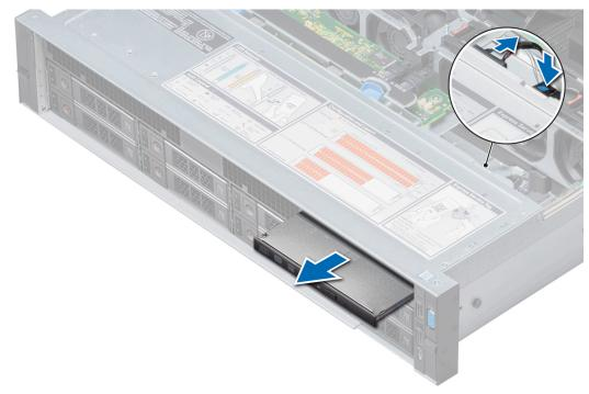
Figure 151. Removing the optical drive
