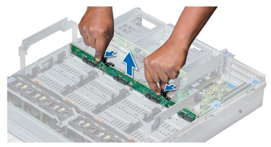
Figure 129. Removing the mid drive tray backplane
