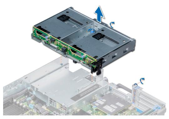
Figure 62. Removing a 2 x 3.5 inch hard drive rear cage
