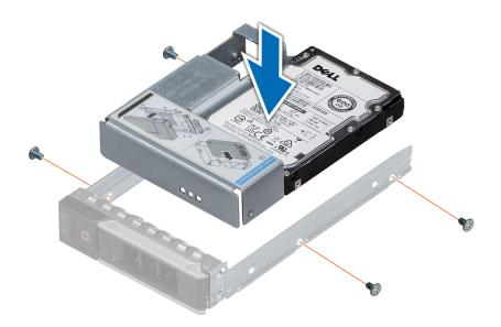
Figure 58. Installing a 3.5 inch adapter into a 3.5 inch drive carrier
