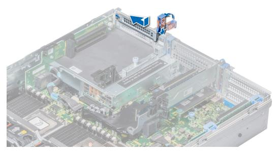
Figure 85. Installing a filler bracket for riser 3
