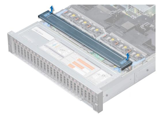
Figure 29. Removing the backplane cover
