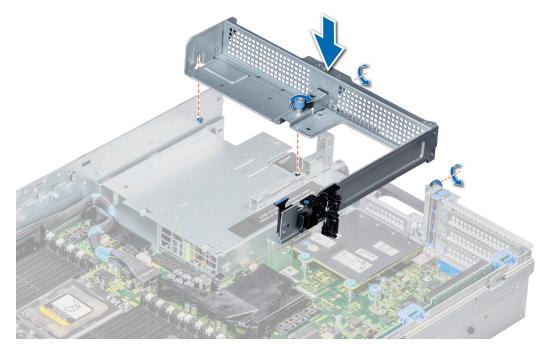
Figure 93. Installing the riser 2 and 3 blank
