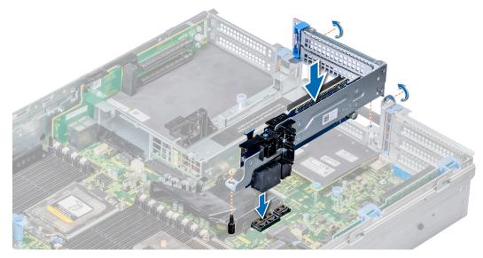
Figure 100. Installing the expansion card riser 2A
