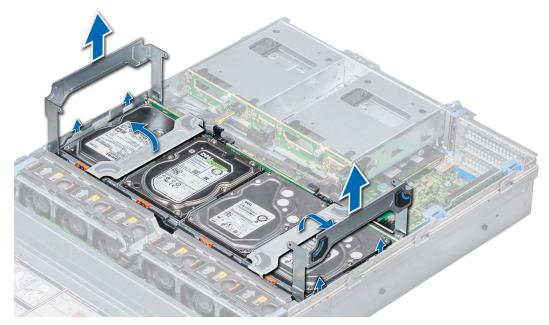
Figure 41. Removing the mid drive tray
