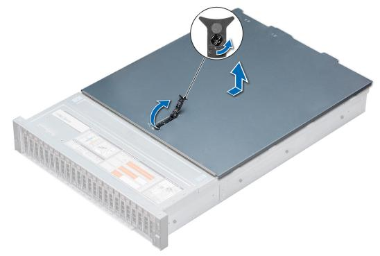
Figure 27. Removing the system cover
