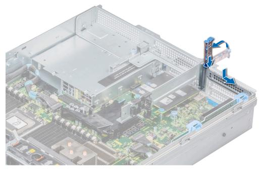
Figure 83. Installing a filler bracket for riser 1
