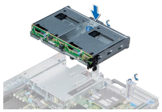
Figure 64. Installing a 2 x 3.5 inch rear hard drive cage
