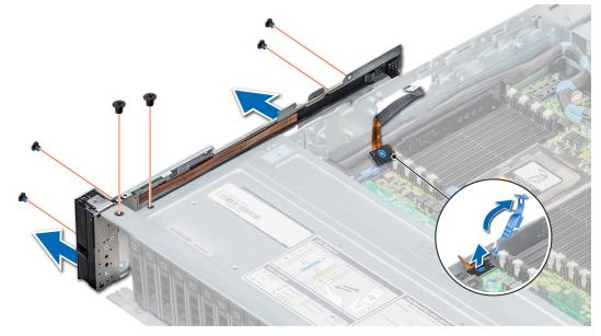
Figure 157. Removing the left control panel
