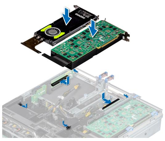
Figure 112. Installing GPU 2 and 3
