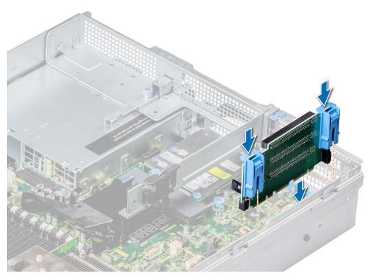
Figure 97. Installing the expansion card riser 1
