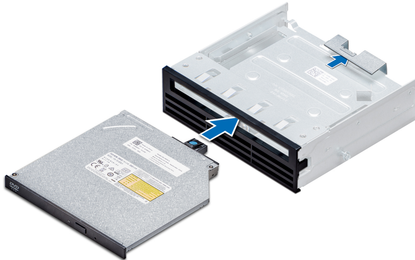
Figure 59. Installing the slim optical drive blank
