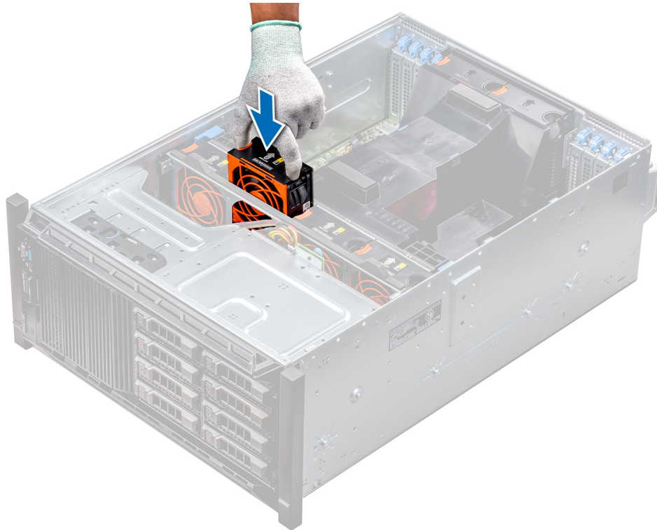
Figure 47. Installing a middle cooling fan
