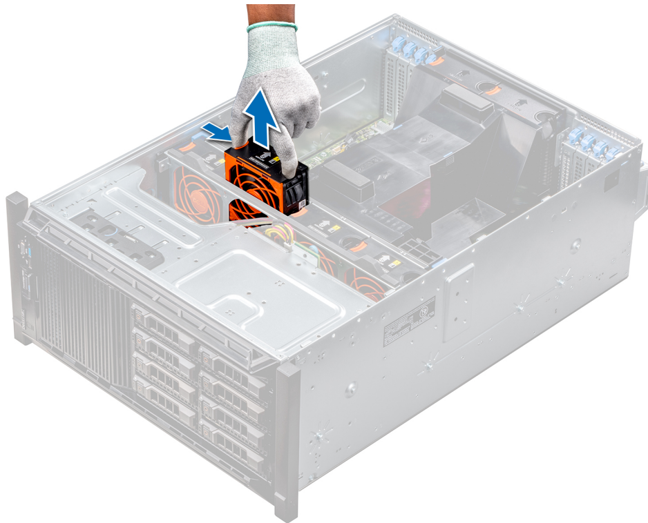
Figure 46. Removing a middle cooling fan
