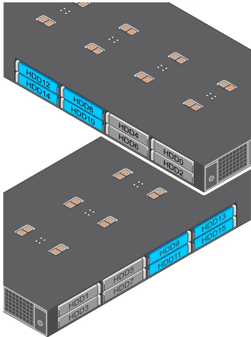
Figure 15. Mapping of drives to dual storage controllers
