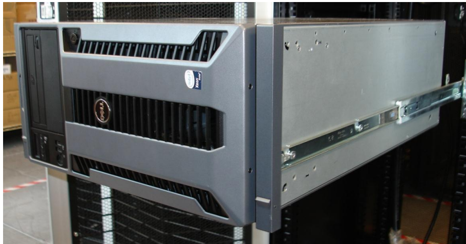
Figure 12. T610 Mounted in C1 Sliding Rails
