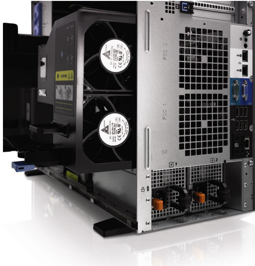
Figure 5. Fans and Cooling Shroud
