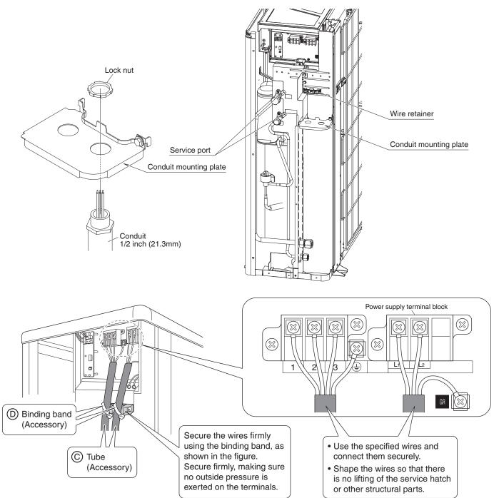
Observe the notes mentioned following when wiring to the power supply terminal block. Precautions to be taken for power supply wiring.
