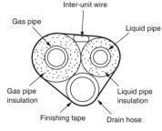
• Use separate thermal insulation pipes for gas and liquid refrigerant pipes.
