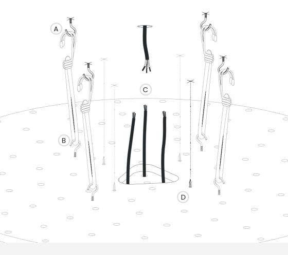
Above is a diagram detailing how the Flock Chandelier is secured to the ceiling and connected to the power supply using the bungees provided to aid installation. The bungees take the weight of the chandelier whilst the electrical connection is being made.
