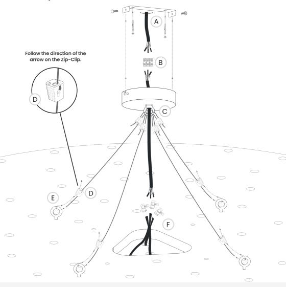
Above is a diagram detailing how the Flock Chandelier is secured to the ceiling rose and connected to the power supply using the tension wires and Zip-Clips provided to aid installation. The tension wires suspend the chandelier but also take the weight of the chandelier whilst the electrical connection is being made.
