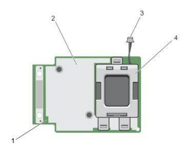
Figure 4. Features of PERC H730/H730P mini monolithic card
