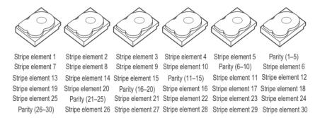
Figure 26. Example of Distributed Parity (RAID 5)
