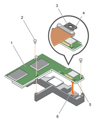
Figure 21. Removing and installing the PERC FD33xD card
