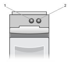
Figure 23. Disk Carrier LED Indicators
