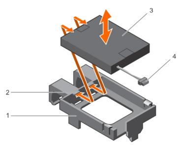
Figure 13. Removing the battery
