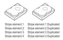
Figure 25. Example of Disk Mirroring (RAID 1)
