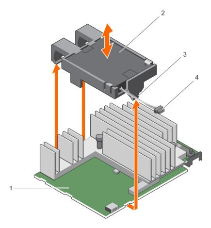
Figure 12. Removing the battery carrier
