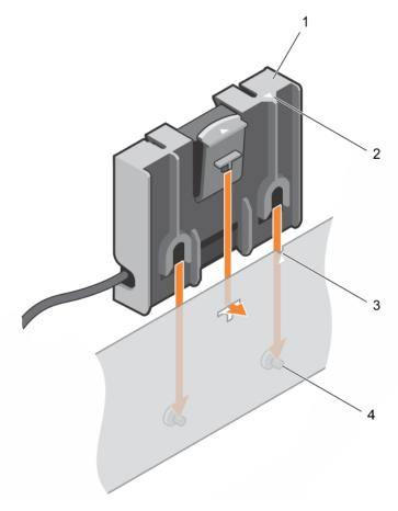
Figure 20. Replacing the battery carrier
