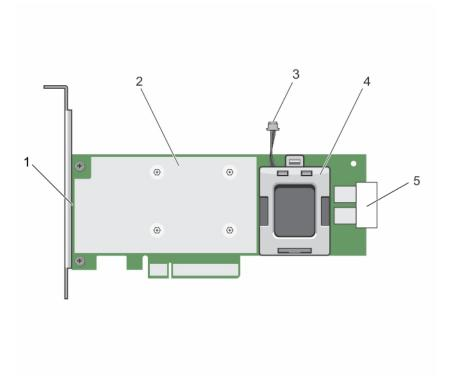
Figure 3. Features of PERC H730 adapter card
