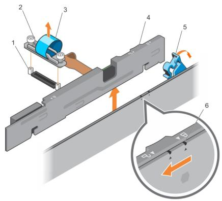
Figure 14. Removing and installing a H730P slim card
