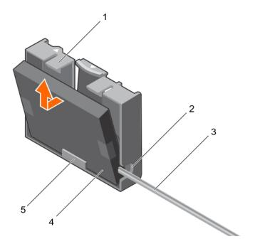
Figure 18. Removing the battery from the battery carrier
