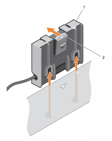
Figure 17. Removing the battery carrier
