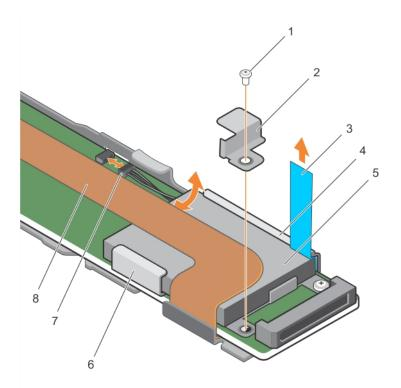
Figure 15. Removing the battery
