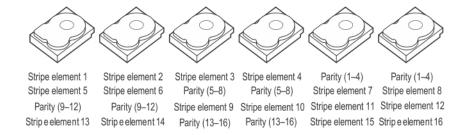
Figure 27. Example of Dual Distributed Parity (RAID 6)
