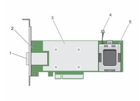
Figure 6. Features of PERC H830 adapter card
