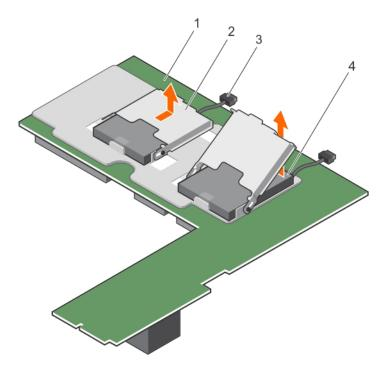
Figure 22. Removing the battery
