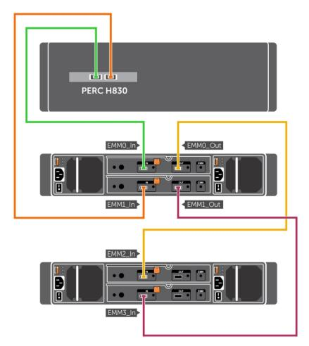
Figure 8. PERC H830 card ports
