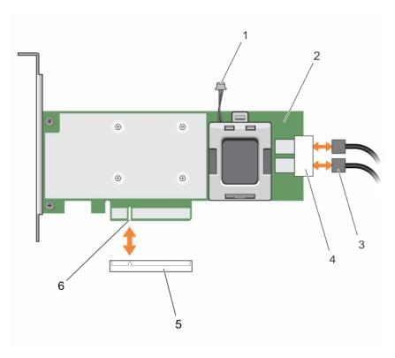
Figure 10. Removing and installing the PERC 9 card
