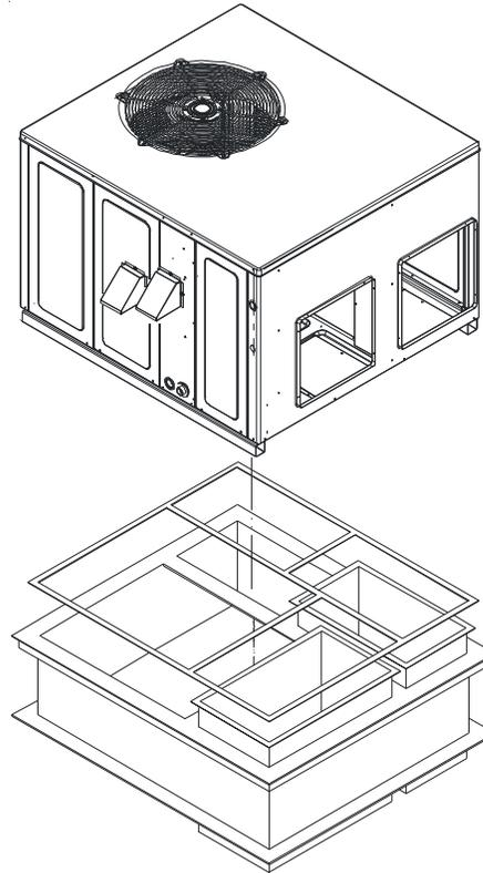
**NOTE:** A roof curb can be used to utilize bottom discharge. APG/GPG Package Units are designed for outdoor installations only in either residential or light commercial applications.
