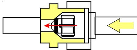
In the cooling mode the orifice is pushed into its seat forcing refrigerant to flow through the metered hole in the center of the orifice.
