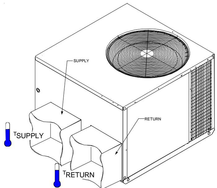
$$\text{RISE} = T_{\text{SUPPLY}} - T_{\text{RETURN}}$$
