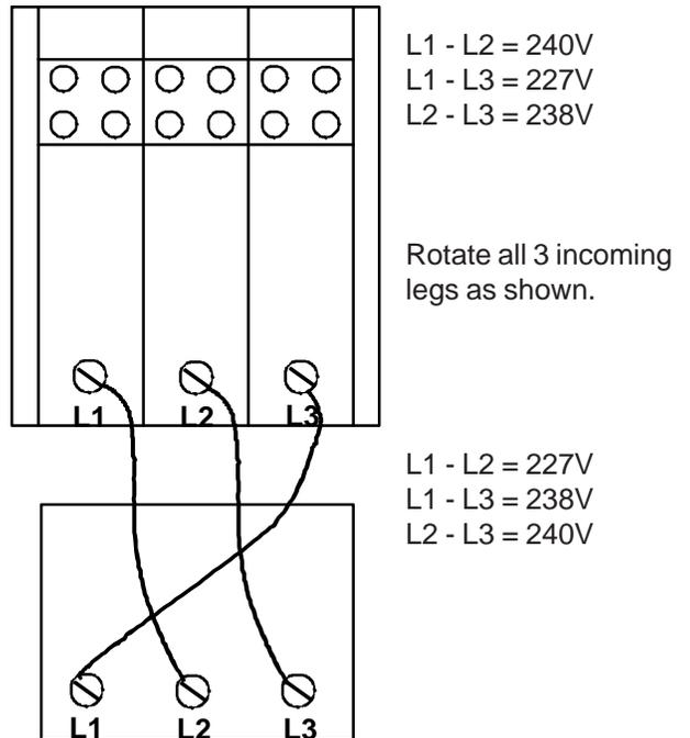
By the voltage readings we see that the imbalance rotated or traveled with the switching of the incoming legs. Therefore the imbalance lies within the incoming power supply.
