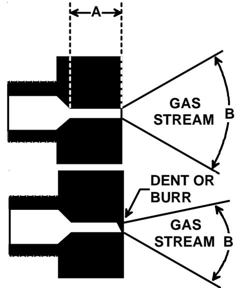
The length of Dimension "A" determines the angle of Gas Stream Defraction, "B".
