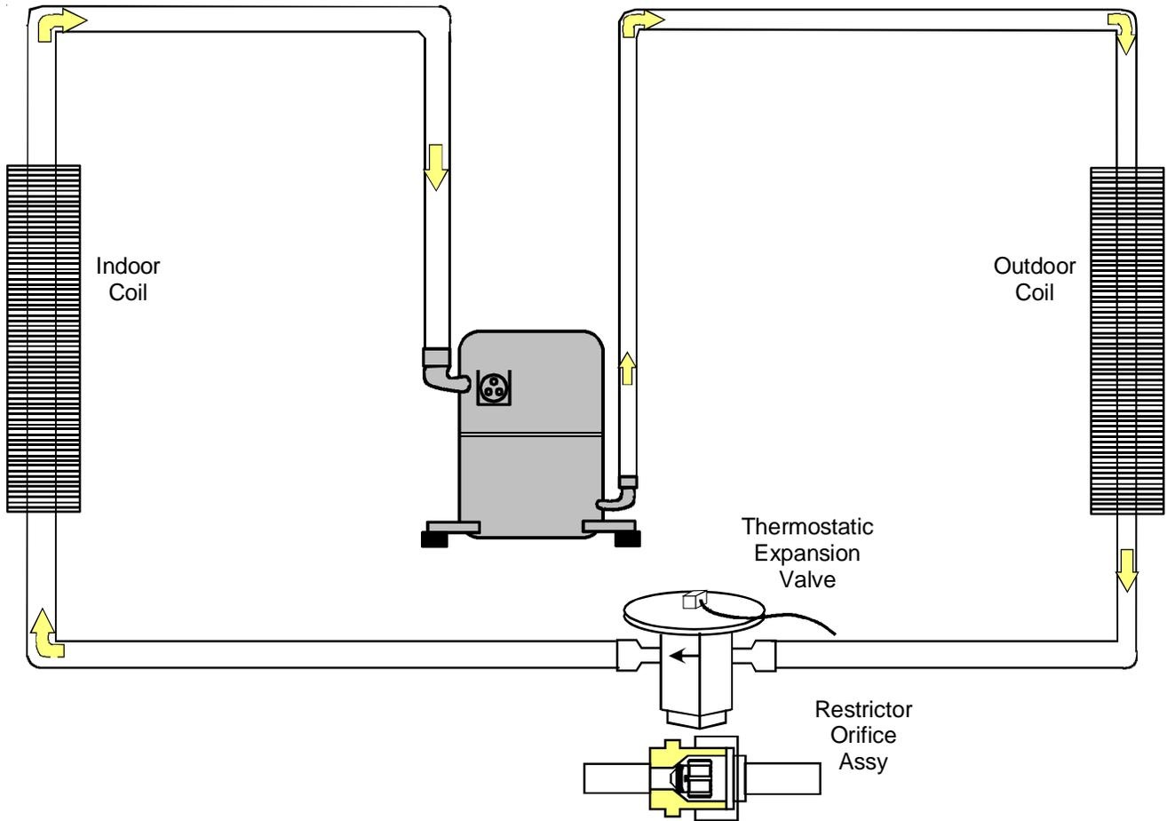
Either a thermostatic expansion valve or restrictor orifice assembly may be used depending on model, refer to the parts catalog for the model being serviced.
