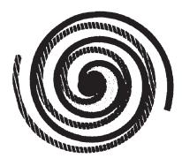
As this motion occurs, the pockets between the two forms are slowly pushed to the center of the two scrolls while simultaneously being reduced in volume. When the pocket reaches the center of the scroll form, the gas, which is now at a high pressure, is discharged out of a port located at the center.
