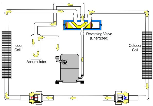
Typical Heat Pump System in Heating
