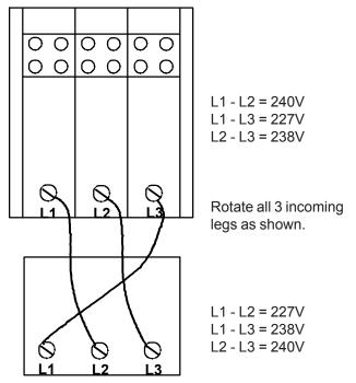
By the voltage readings we see that the imbalance rotated or traveled with the switching of the incoming legs. Therefore the problem lies within the incoming power supply.
