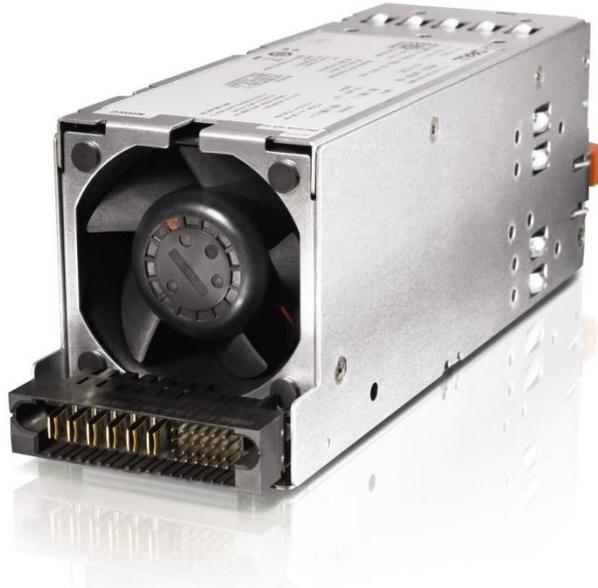
Dell power supplies use output ORing FETs to isolate the power supply from the 12V system bus. If a single power supply fails its output ORing FET, the power supply will turn off removing itself from the bus like an electrical switch that turns off when the power supply fails.
