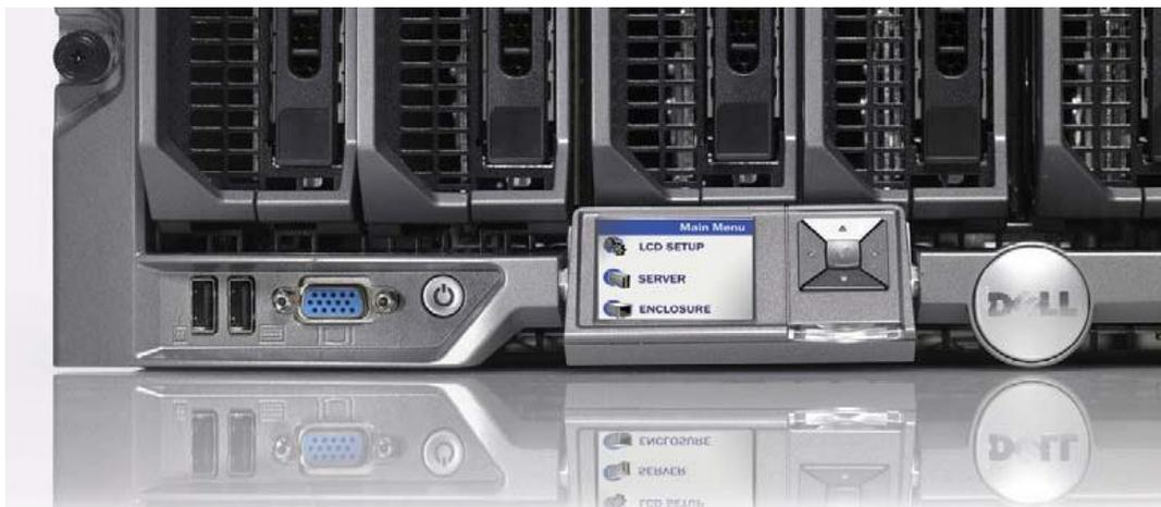
The LCD panel can be used as a diagnostic source and as a place to configure parameters of certain chassis components as well as the server's iDRAC with Lifecycle Controller network configuration. The primary function of the LCD panel is to provide real-time information on the health and status of the modules in the enclosure. LCD panel features include:
